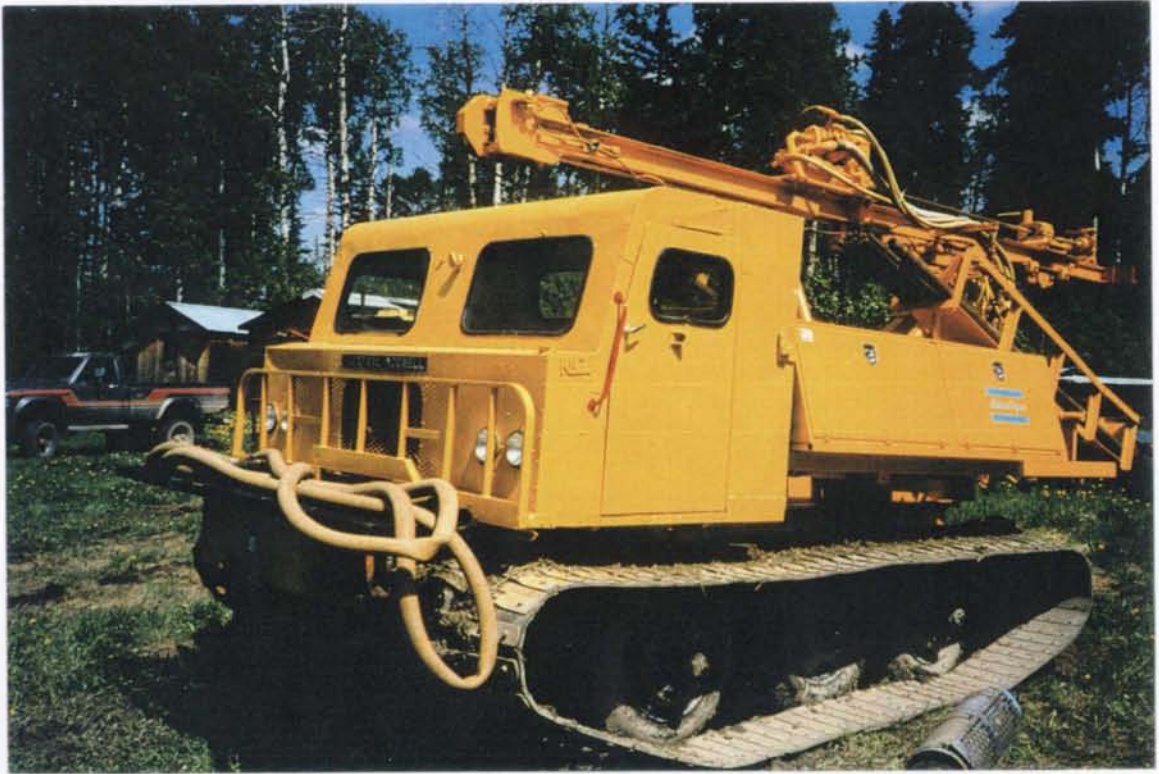
Plate 1: Nodwell mounted Atlas Copco BRE 5701
