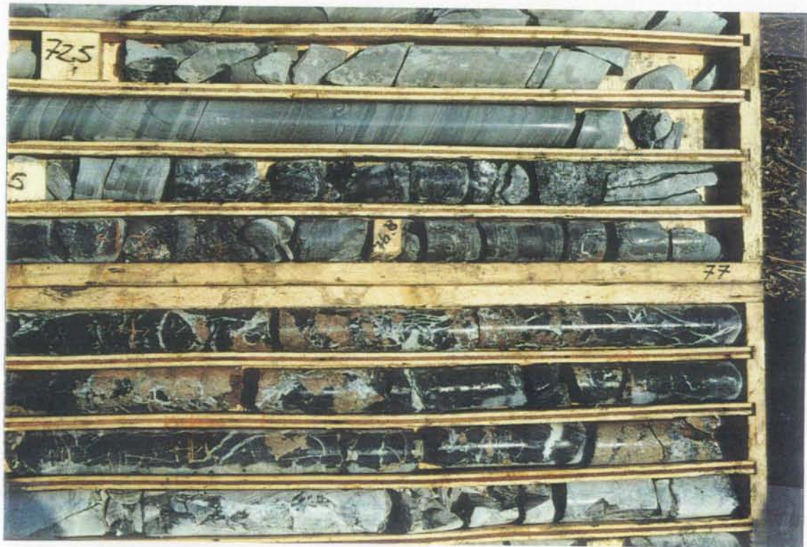
Hole No. J-95-4 From 69.5-84.2 m Thin bedded calcareous siltstone overlies black sphalerite-rich chert; massive Cryptograined Limestone underlies the mineralized chert
