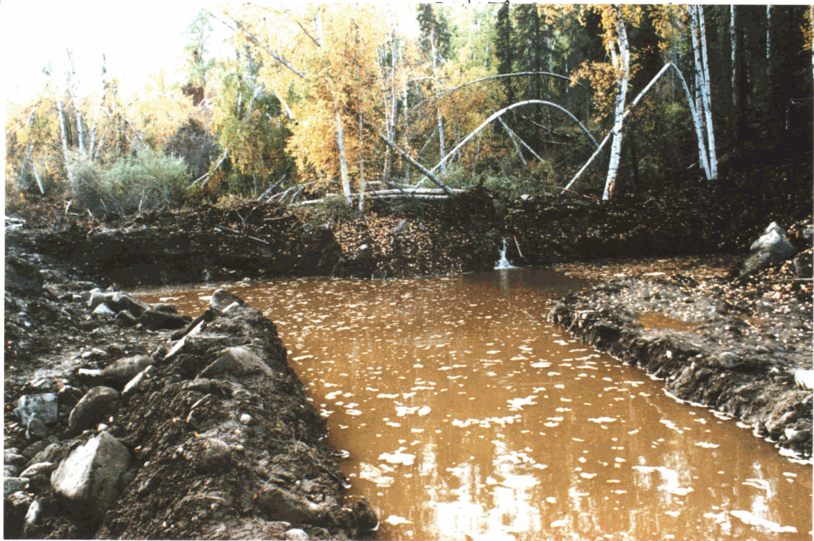
1987 TEST PIT (PL26859) IN HIGH GRADE PLACER (FLOODED RAMP IN FOREGROUND BEGINS AT 15' DEPTH AND LEADS TO CAMERA. TEST SLUICE BEHIND PHOTOGRAPHER)
