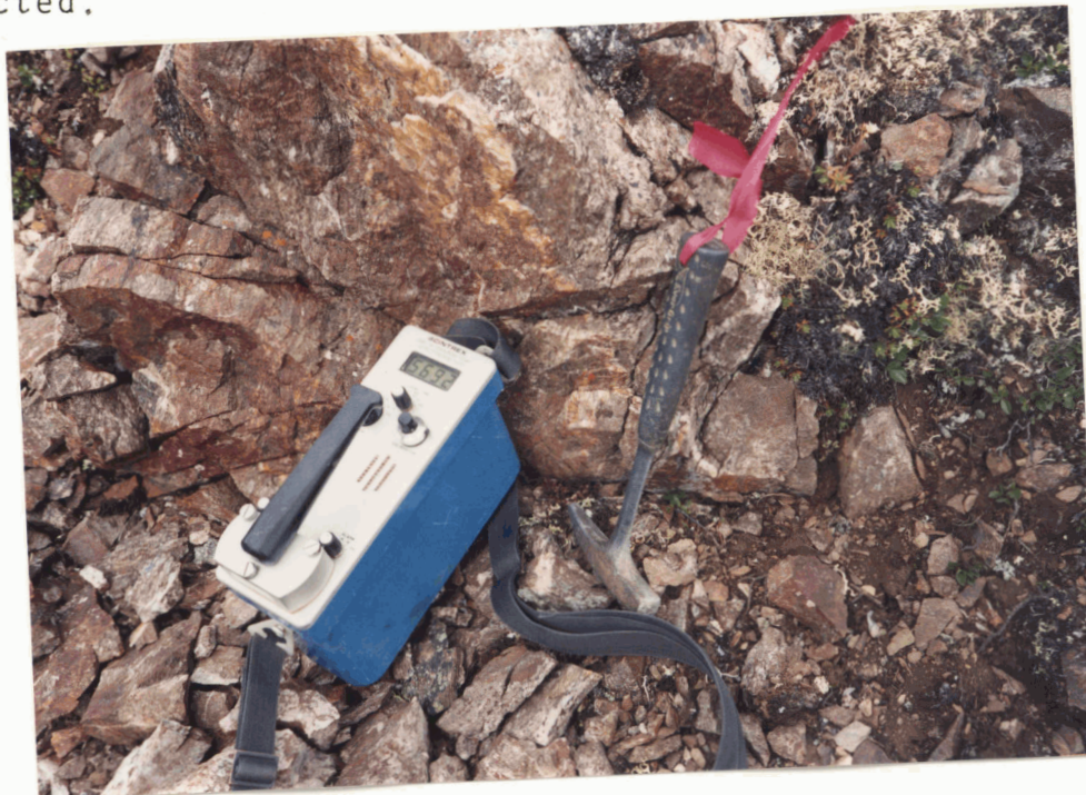
Radiometric scanning using a GIS-4 gamma ray spectrometer to identify outcrops mostlikely to contain yttrium, zirconium, and REE owing to high radioactivity signatures from accompanying thorium and uranium minerals.
