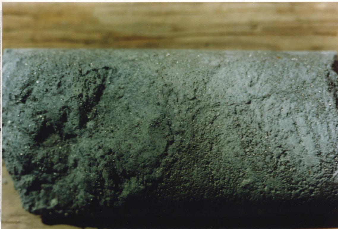
PHOTO 3. PYRITE MINERALIZATION RWS 89-1, FROM FAULT ZONE SECTION 41.57 - 42.06 METRES, ASSAYING 0.546 OZ/T GOLD
