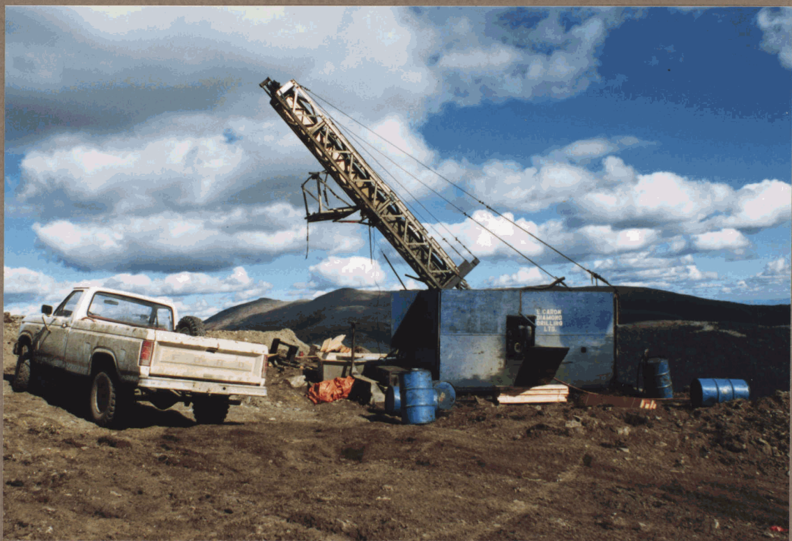
6. Diamond drill set up on Hole 86-9, ORO property, Yukon.
