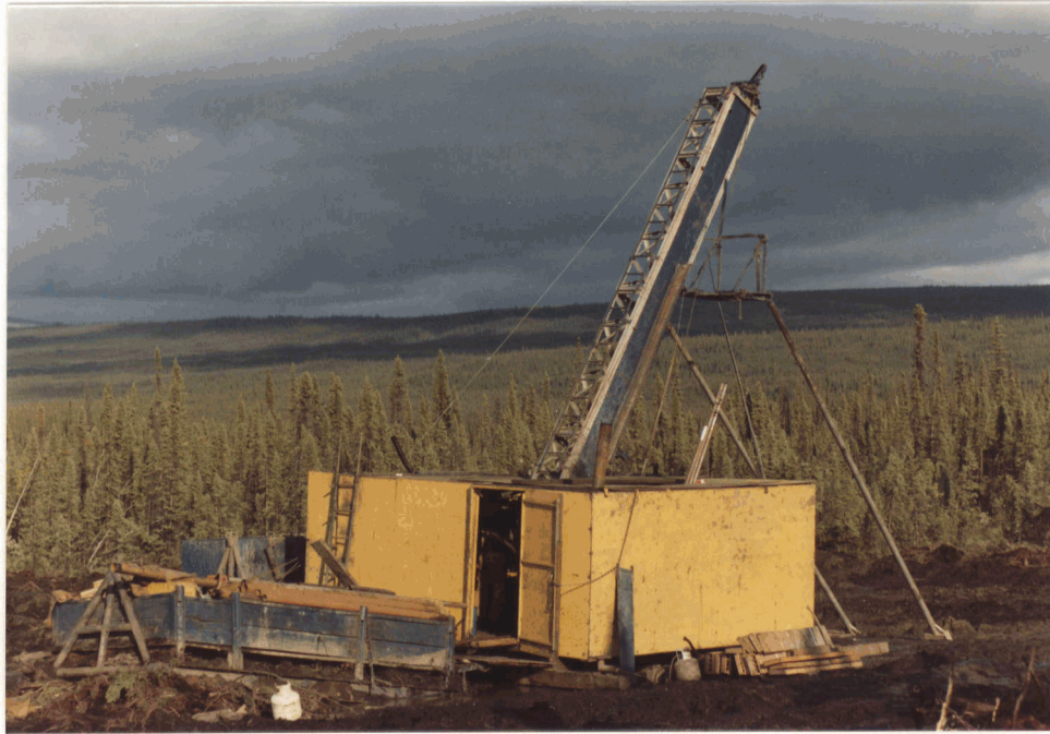
Longyear Super 38 diamond drill rig on hole DDH-81-01B
