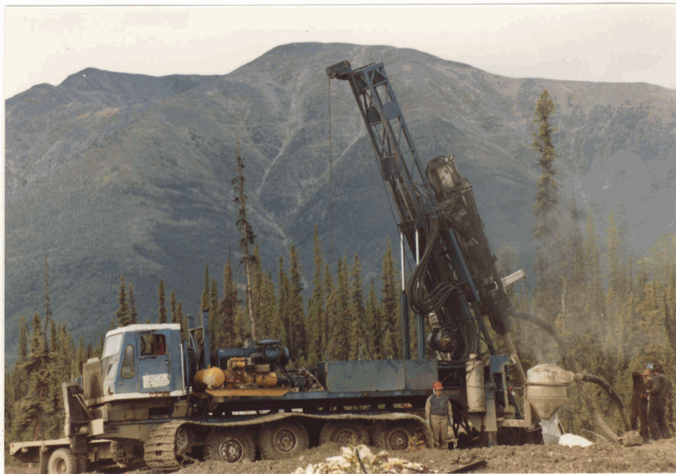
Becker 180 hammer drill mounted on a nodwell, on hole 81-02A
