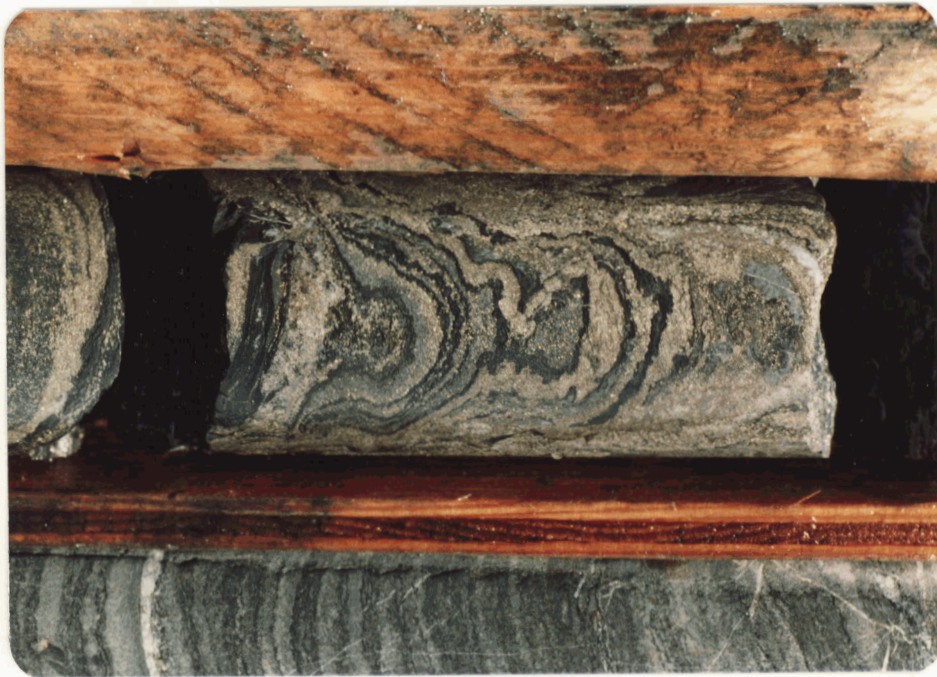
Figure 3. type 3 sulphides coarsely crystalline "disturbed" sulphides consisting of pyrite and pyrrhotite with lesser chalcopryrite, sphalerite and galena Cord claims, DDH 81-1.
