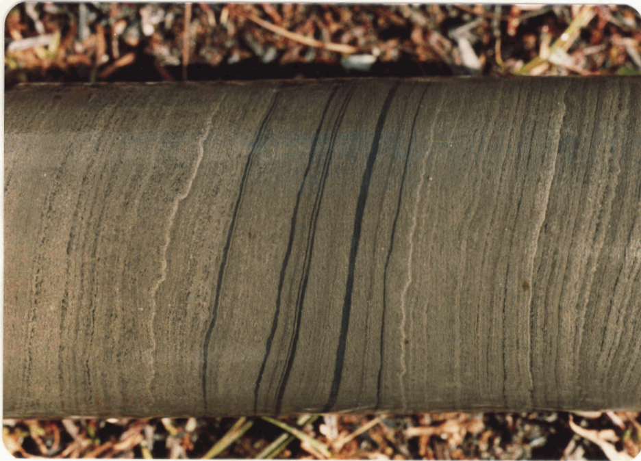
Figure 2. type 2 sulphides-finely crystalline laminated pyrite and pyrrhotite with minor sphalerite galena and chalcopryrite; note graded beds and minor folds, Cord claims, DDH 81-1.
