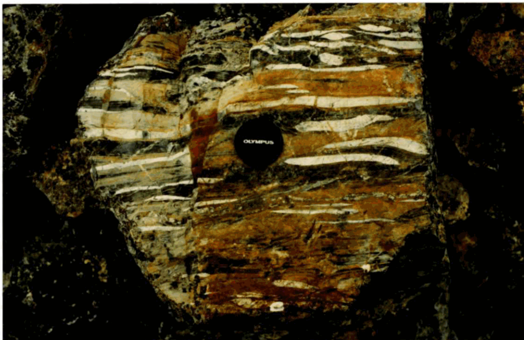
Plate # 2. "Zebra" rock, western intrusive complex. Interbedded chert, white cherty siltstone and argillite.
