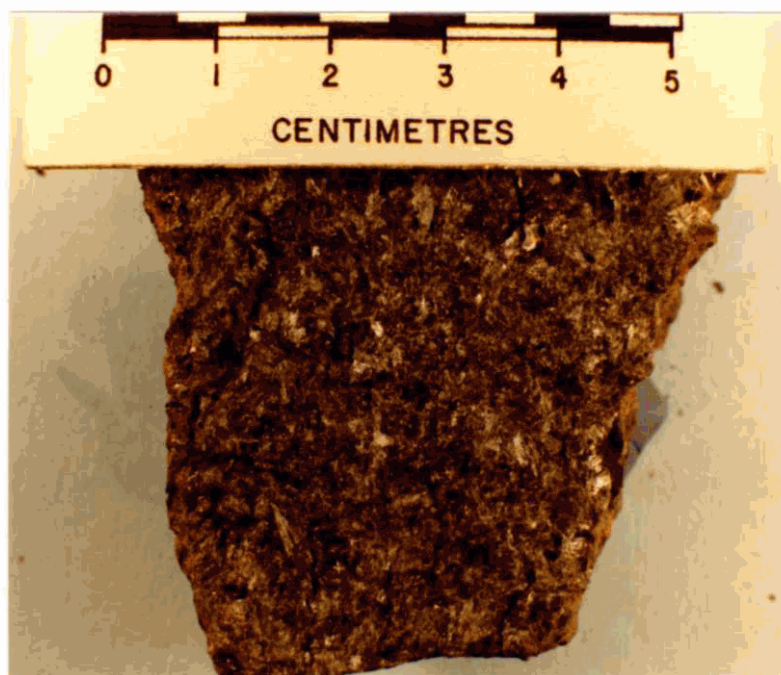
Figure 3. Biotite pyroxenite (BI PXNT) from the VAL mafic-ultramafic suite. Biotite content (0-30%) is the only visible difference between pyroxenite and biotite-pyroxenite.
