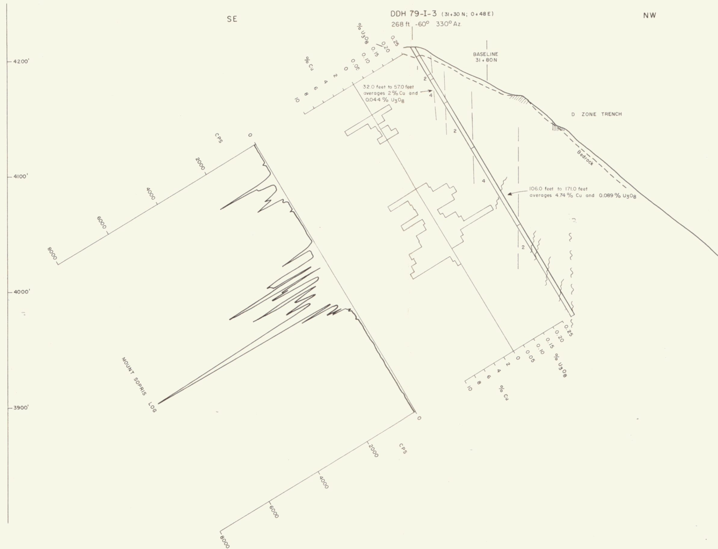
Figure WJV79-I5 ARCHER, CATHRO & ASSOCIATES LTD CROSS-SECTION HOLE 79-I-3 IGOR CLAIMS WERNECKE JOINT VENTURE Scale 1:600 (1 Inch = 50 Feet)
