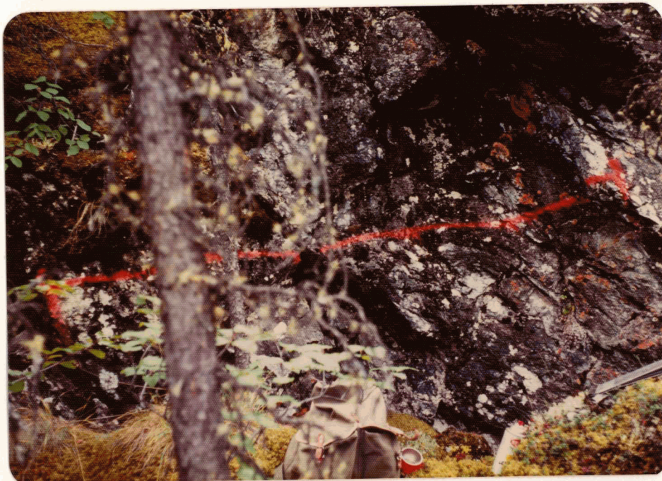
Photo 2 - Showing on south west portion 'A' grid - 8' chip sample.
