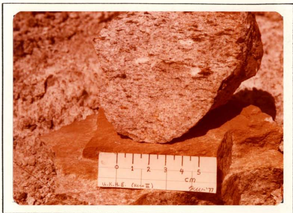
PHOTO 5. Fine-grained strongly foliated granitic rock from the southeast end of Zone 1. Limonite specks may indicate weathered sulphides or mafics. - K.W.
