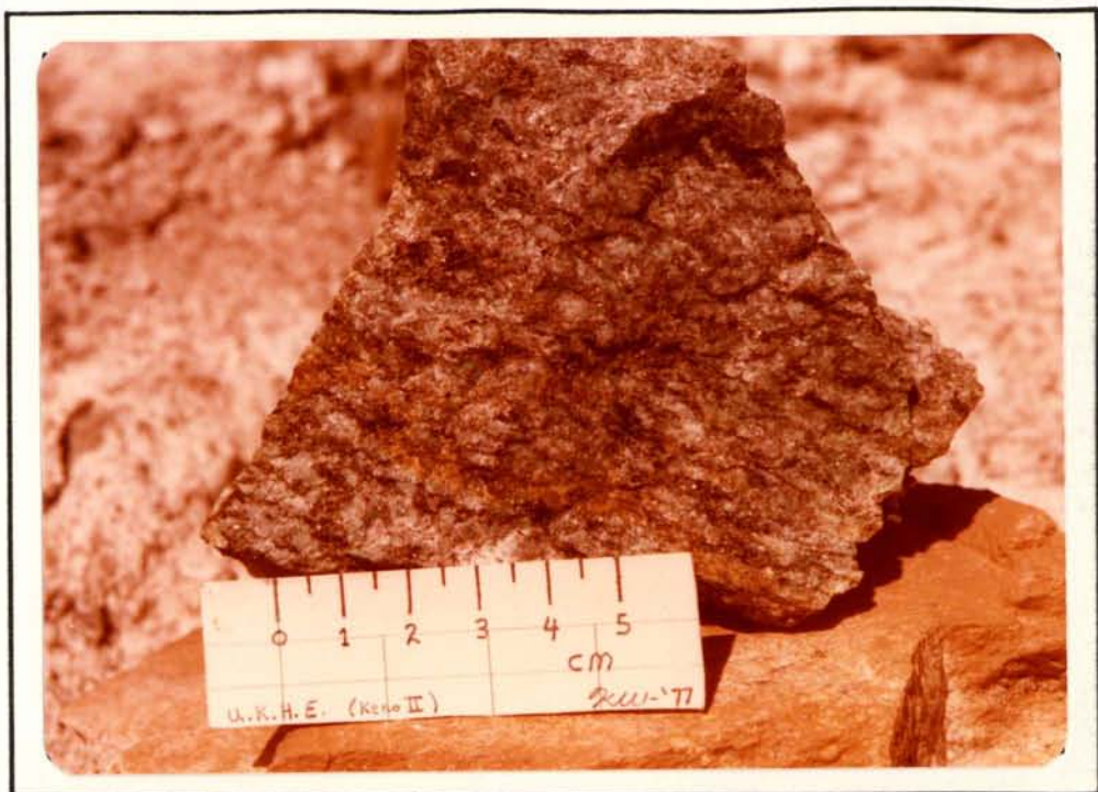
PHOTO 3. Malachite impregnated strongly foliated hornblende-biotite granodiorite from the central part of Zone 1. - K.W.
