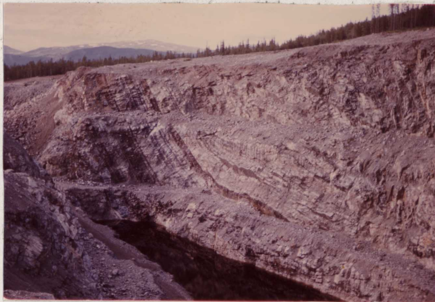
Plate #7 Interbedded anhydrous skarn and carbonaceous sediments in the War Eagle pit.
