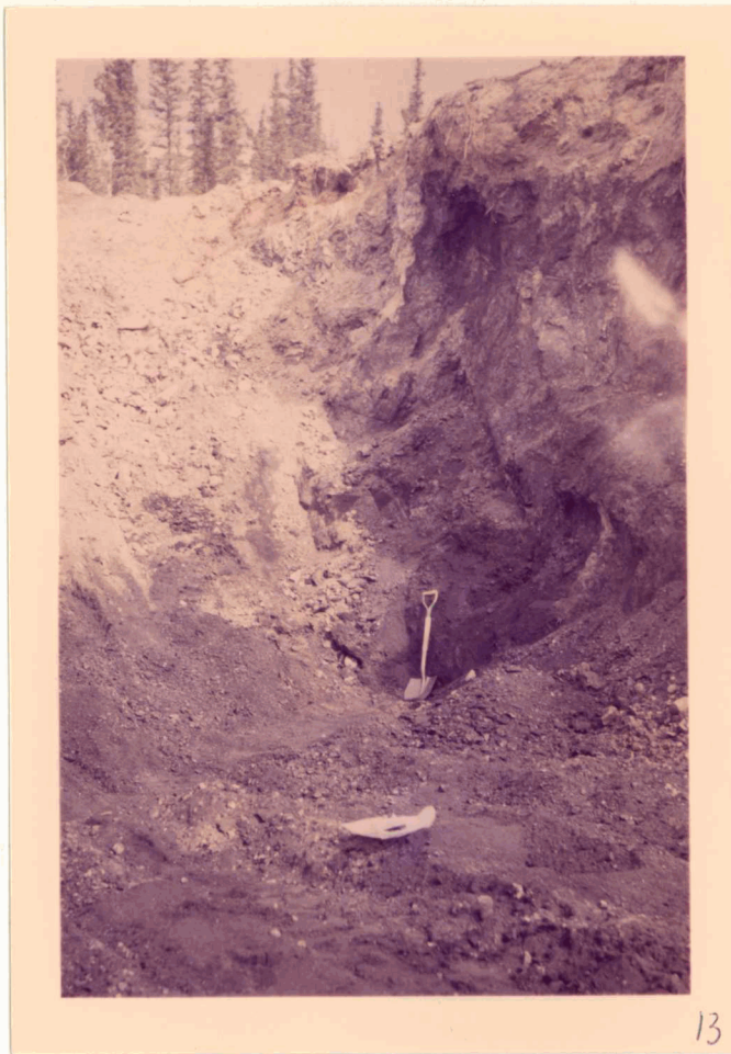
Photo No. 13 - Pit No. 2 Sampling Seam 'F' Sample #4 taken at shovel.
