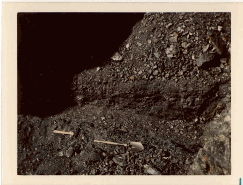
PLATE 7. Trench 5, southwest end in shadow. Trench dump material exhibits high lustre typical of the trench-exposed graphitic anthracite bedrock.
