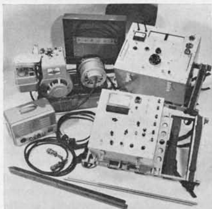
Figure 3.—(above)—The Seigel Mk V Induced Polarization Unit.
