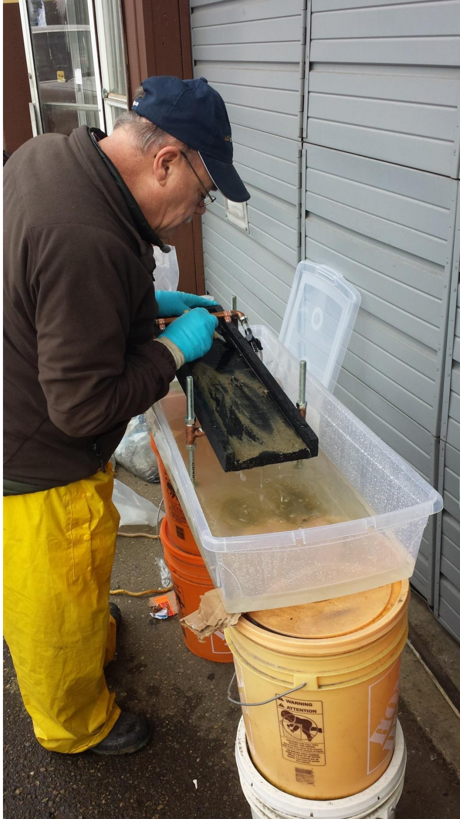
Photo 5 Final Screening, Panning and Microsluice of Heavy Concentrates
