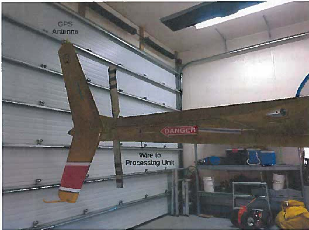
Figure 5: GPS Unit on Helicopter Tail
