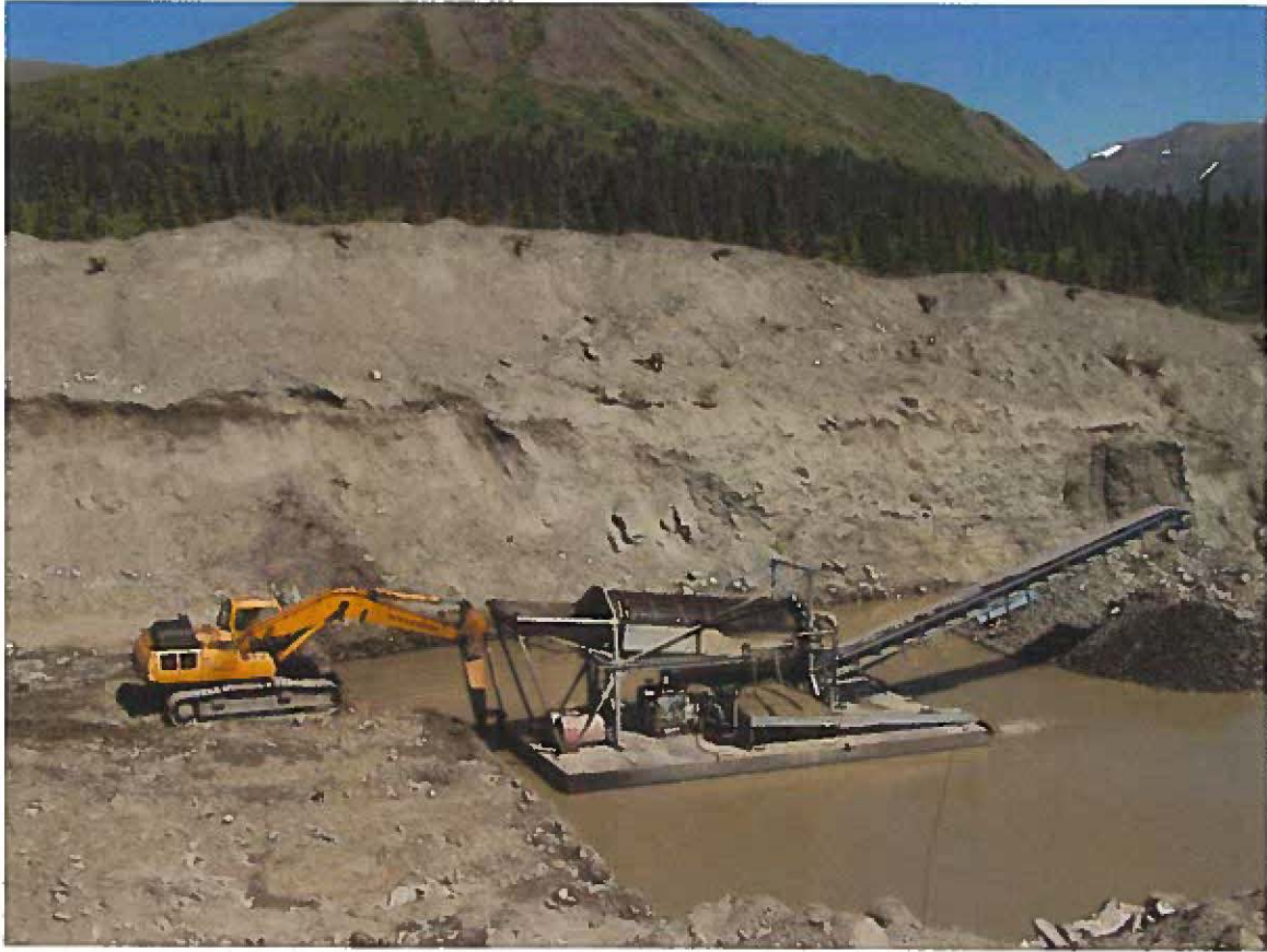
Plate 2 - The washplant and stratigraphic section of the Sota Computing Ltd. operation on the left limit of Fourth of July Creek, 2002. The stratigraphic section consisted of mixed sand and gravel over a layer of glaciolacustrine silt and clay. These sediments were above a pay gravel which was floored by a "false bedrock" of glacial till.
