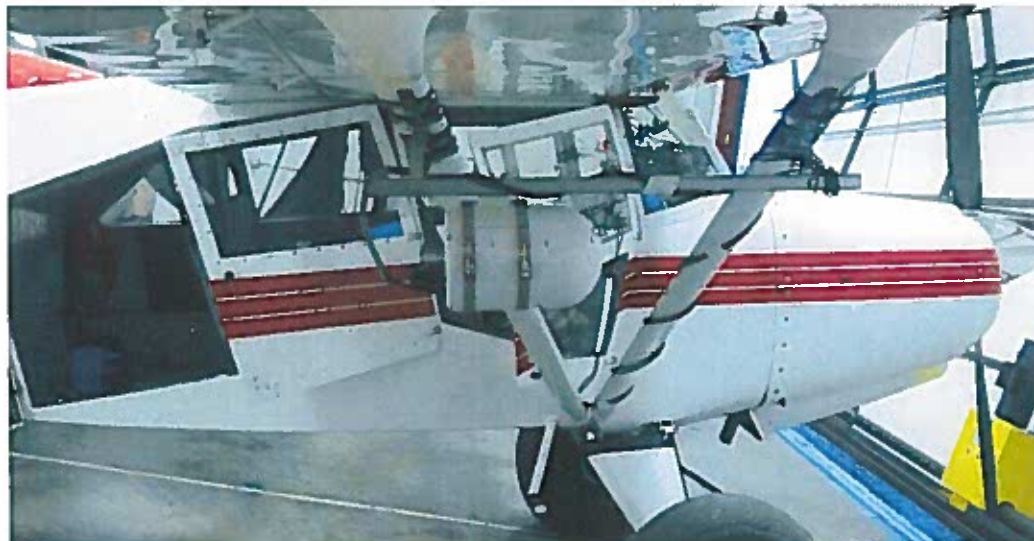
Figure 3. The pod secured the bar attached to the strut.
