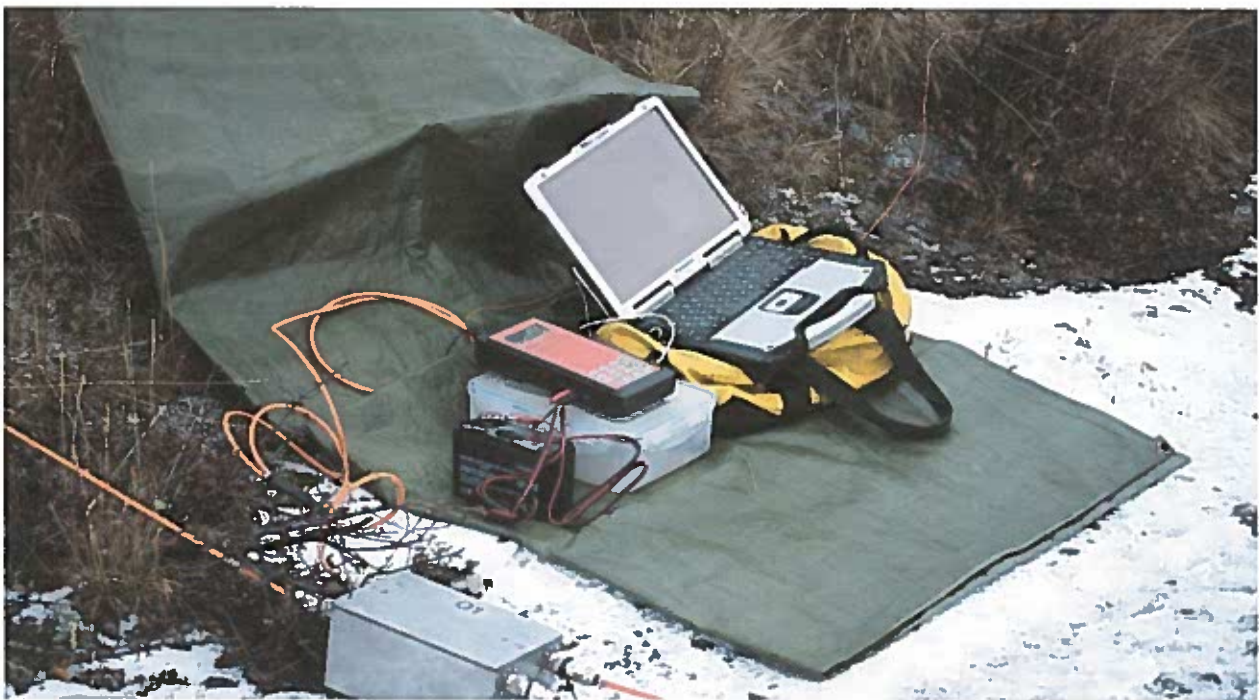
Figure 2 : 2D Resistivity measurement, Stefan Ostermaier, Arctic Geophysics Inc., Atlin, BC 2013
