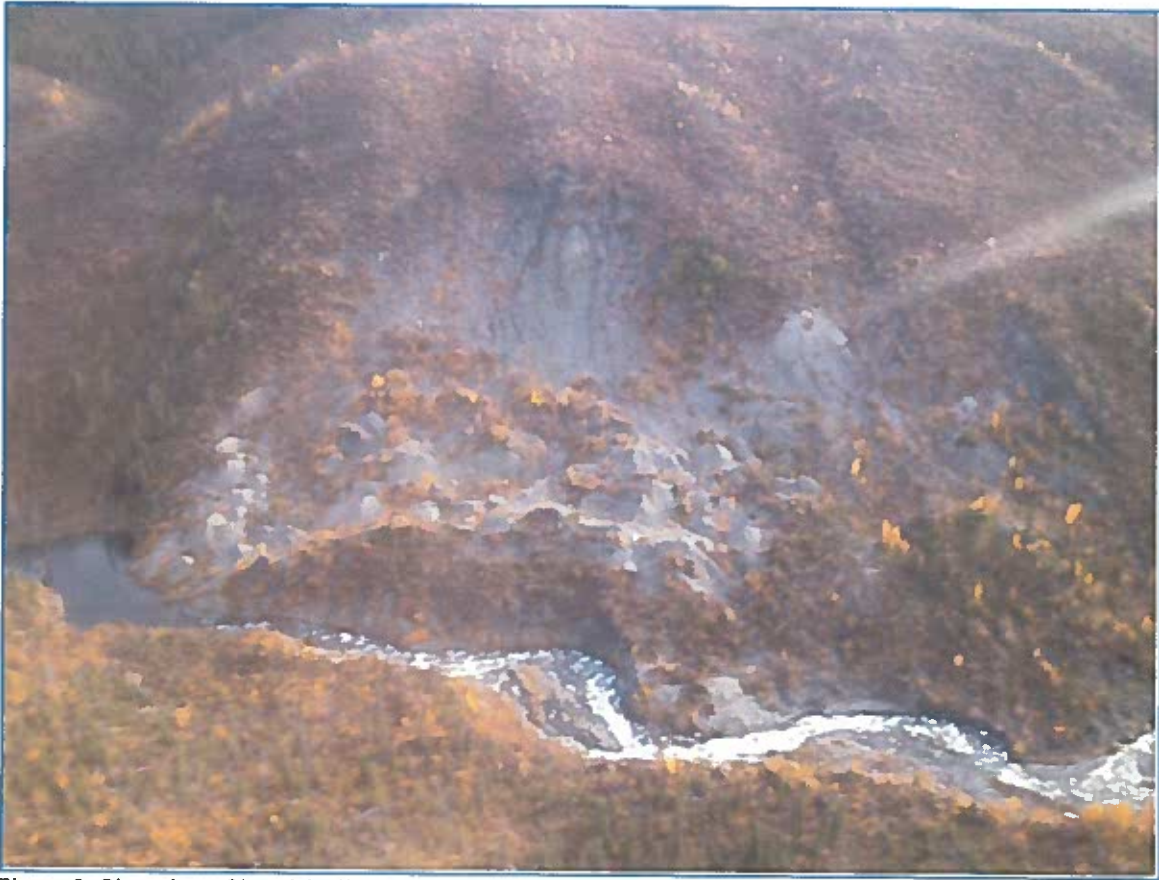
Figure 3. Slumping of ice-rich silty till in terminal moraine.
