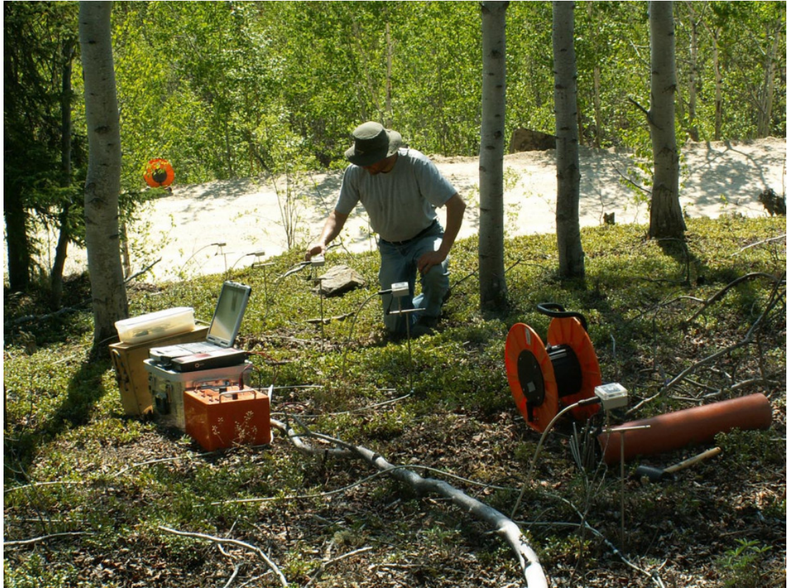
Figure 01: 2D Resistivity/IP measurement, Stefan Ostermaier, Arctic Geophysics Inc., Yukon 2009 (Moll)
