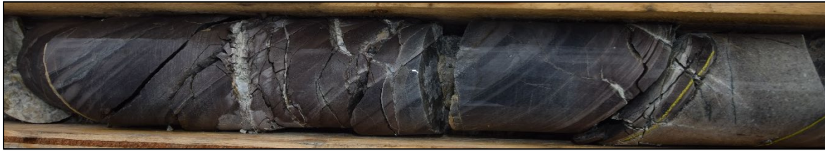
Plate 1 - Laminated siltstone, Yusezyu Formation. DDH JN19020: 70.5 m.
