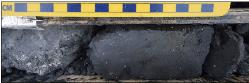
Plate 8 – Type photo of an intensely altered shear zone. DDH JN19021: 210.2 m.
