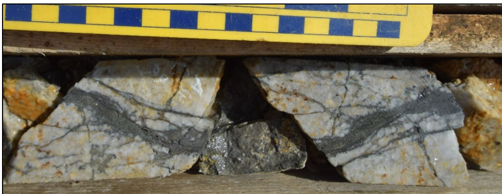
Plate 6 – Semi-massive sulphide mineralization of quartz-carbonate veinlets hosted in quartz-pebble conglomerate, Yusezyu Formation. DDH JN19021: 19.2 m
