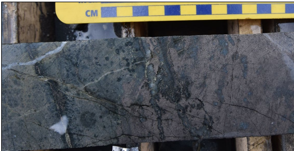
Plate 9 – Semi-massive sulphide (pyrrhotite-pyrite ± chalcopyrite) of pyroxene-rich skarn. DDH JN19021: 250.1 m.
