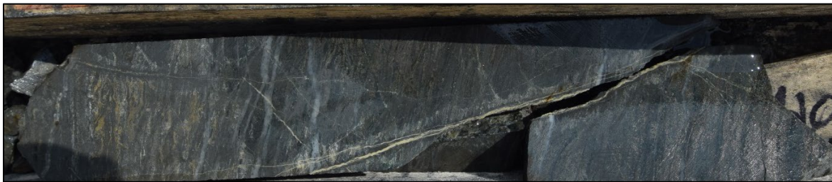
Plate 3 - Semi-massive to massive sulphide replacement of skarn, Yusezyu Formation. DDH JN19020: 167.7 m.
