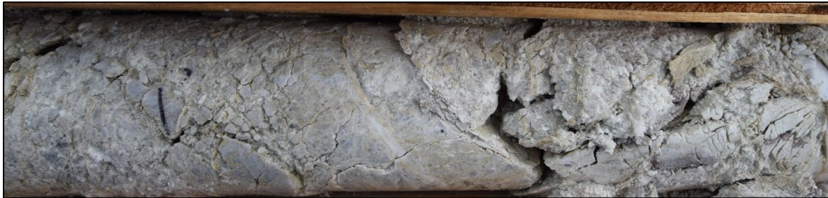
Plate 2 - Partially clay altered Quartz Pebble Conglomerate, Yusezyu Formation. DDH JN19020: 71.0 m.
