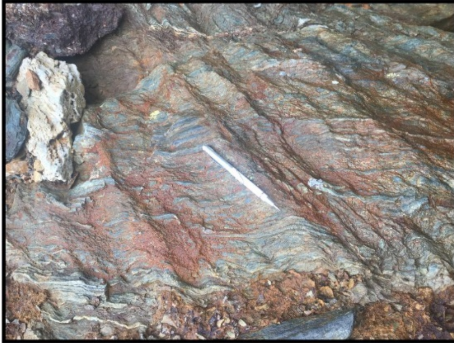
Figure 12: F2 fold axes on S1 foliation surface. The “ribbed” lineation is the bedding/cleavage intersection lineation which has been folded about F2. Darker bands are magnetite alteration which are common near the Kona massive sulfide surface exposure.
