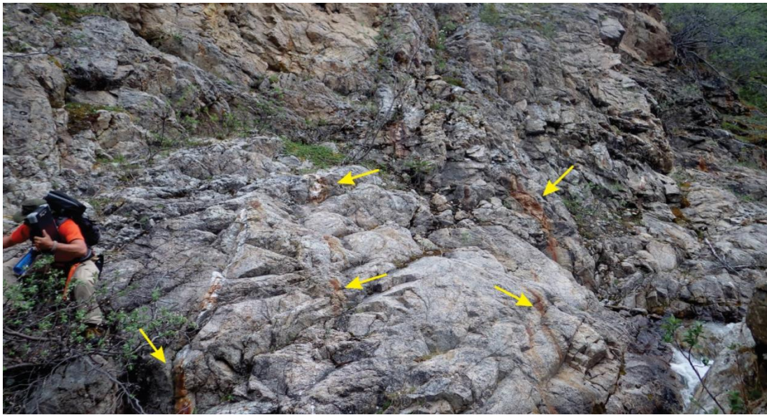
Illustration 3: Rust bleeds depicted by yellow arrows. Field assistant for scale
