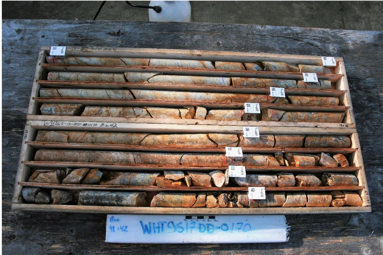
Figure 19: Box 41 to 42 of WHTGS17DD-0170 showing intense quartz carbonate alteration and strong oxidation along fracture seams.
