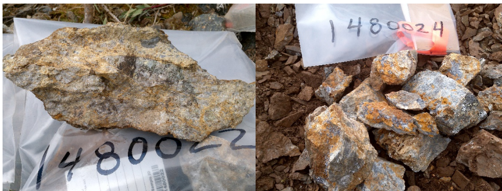
Photo Plate 2. LEFT: Unmineralized sample of the silica-healed breccia. RIGHT: Mineralized sample of the same unit
