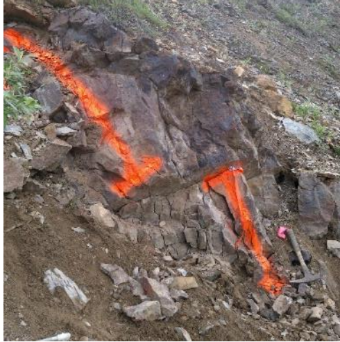
LEFT Photo-plate 3. Hanging wall (1480010) and footwall (1480011) channel samples of skarn-type mineralization. RIGHT Photo-plate 4. Channel sample 1480012 and 1480013 of skarn-type mineralization with visible copper oxide coating below dioritic dyke.
