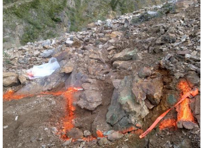
LEFT Photo-plate 3. Hanging wall (1480010) and footwall (1480011) channel samples of skarn-type mineralization. RIGHT Photo-plate 4. Channel sample 1480012 and 1480013 of skarn-type mineralization with visible copper oxide coating below dioritic dyke.
