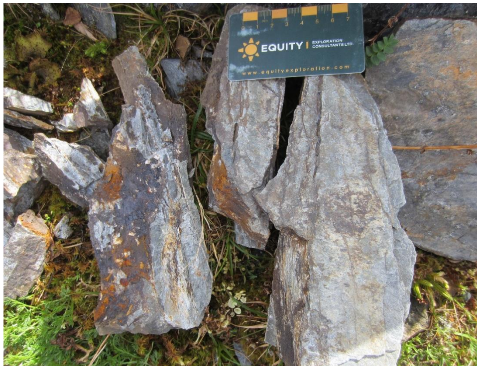
Plate 8: Sample S193113, in float at the north end of North Star soil anomaly. Strongly fractured quartzite with manganese and iron oxides in fractures, weak sericite and silica alteration (459010E/7083965N).
