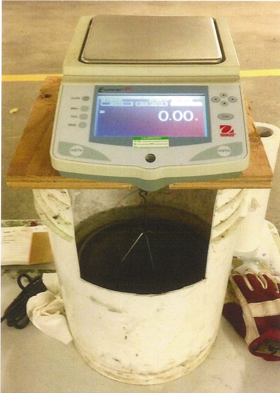
Figure 11. Balance scale and water bucket setup for measuring specific gravity of core
