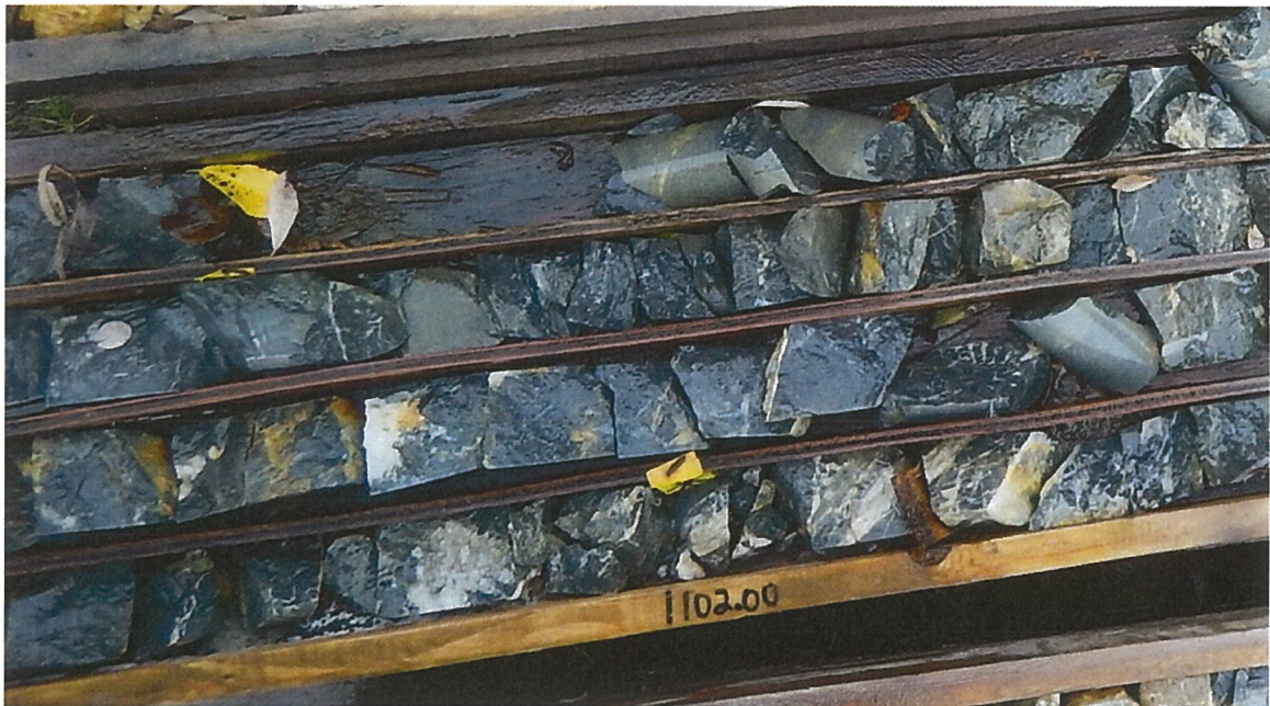
Figure 10. Typical competent drill core sampled for SG test work
