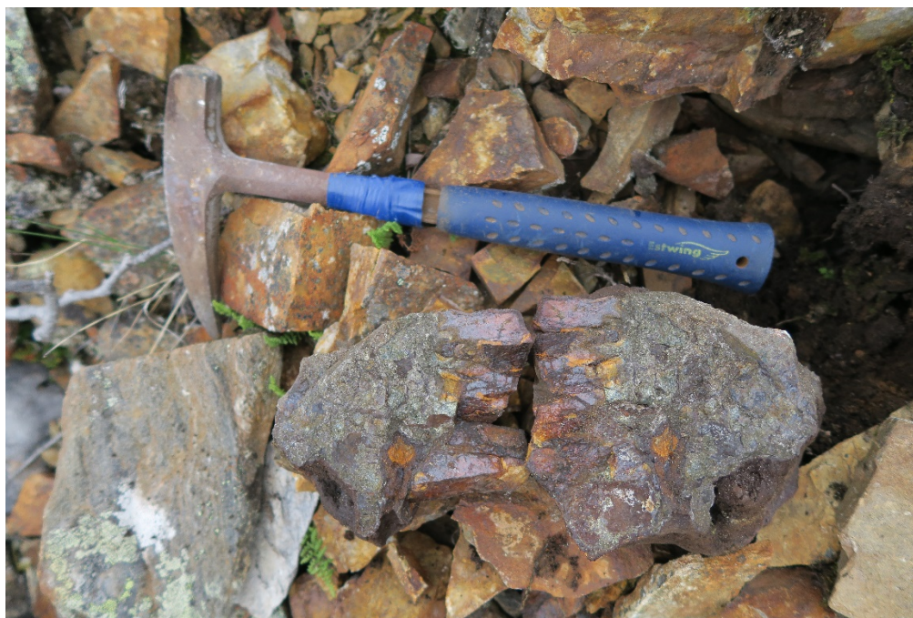
Figure 8: Skarn-hosted, massive sulphide sampled at Charon. Assays returned 36g/t Au, 0.725% Cu, and 17.1g/t Ag (Sample # V177091)
