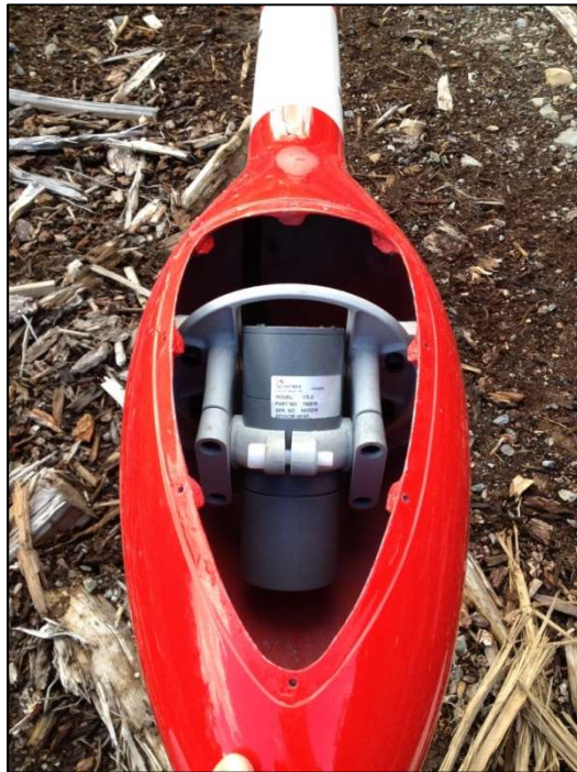
Figure 15: View of cesium vapor magnetometer. Sensor oriented 45° from vertical to couple with local magnetic field at the Golden Horseshoe survey block.
