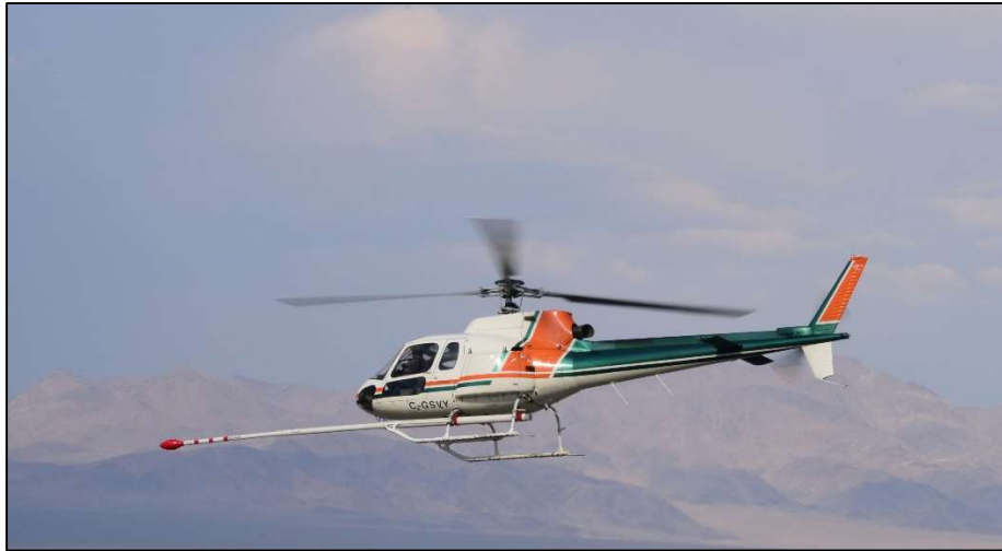
Figure 14: View of magnetic “stinger” installation on survey helicopter.
