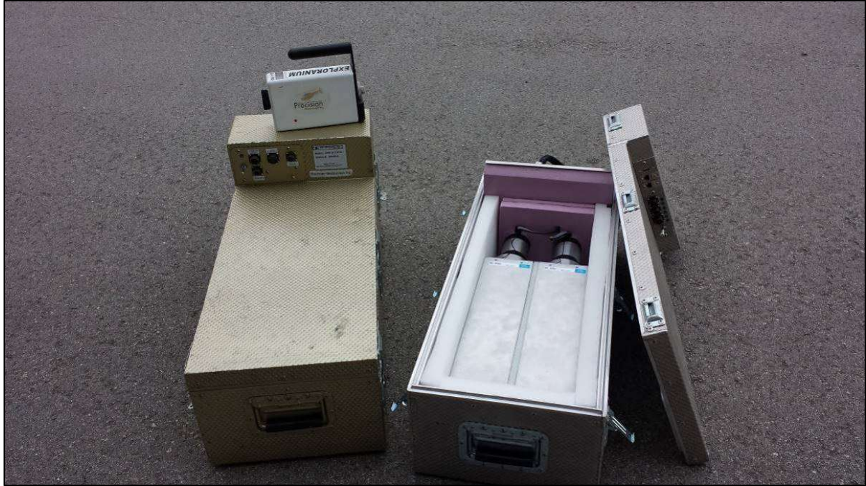
Figure 16: GRS-10 thallium-activated sodium iodide gamma spectrometer crystal packs. The open unit on the right shows two individual 4.2 litre gamma detectors.
