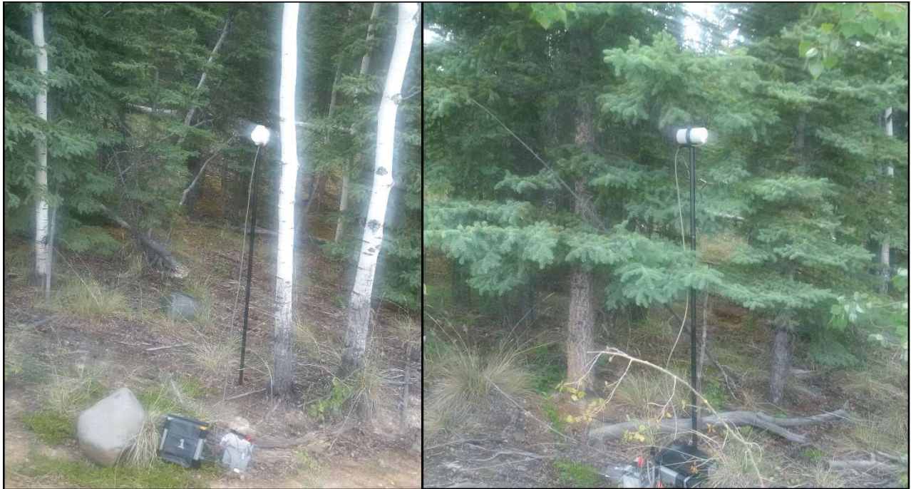
Figure 8: GEM 1 (left) and GEM 2 (right) magnetic base stations located in the bushes at Carmacks airport, Yukon.
