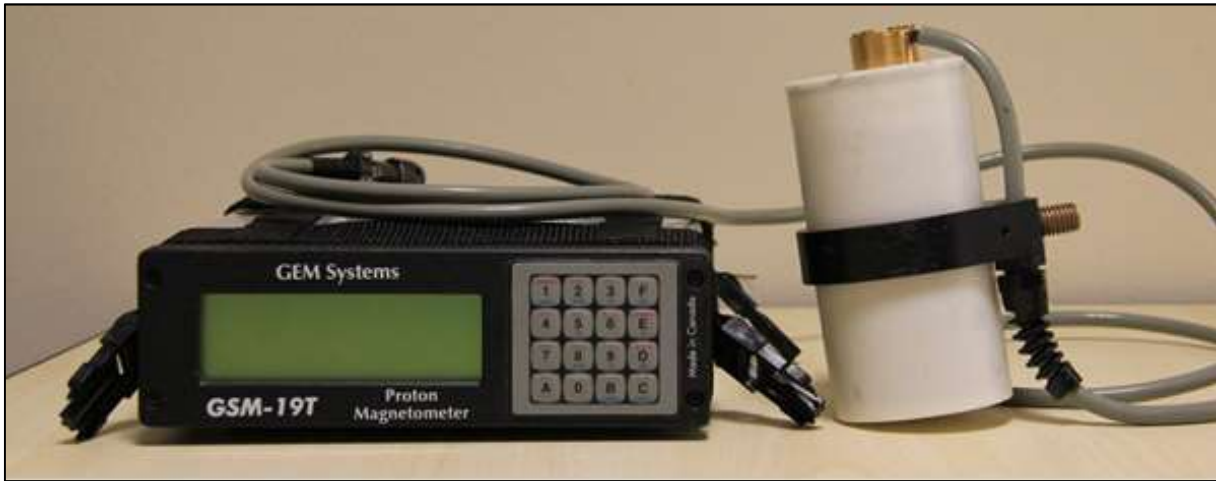
Figure 17: GEM GSM-19T proton precession magnetometer.
