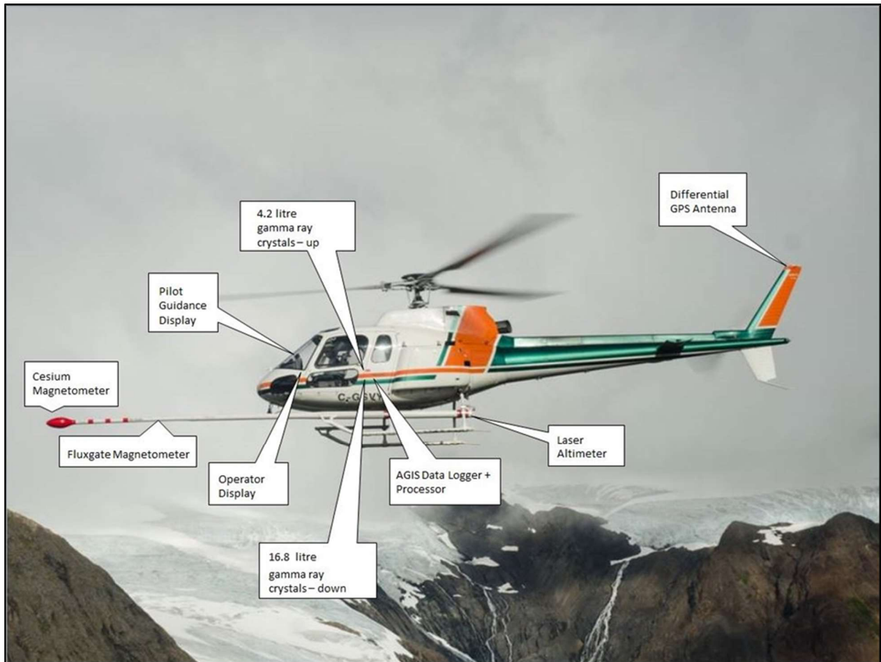
Figure 12: Survey helicopter equipped with geophysical equipment.
