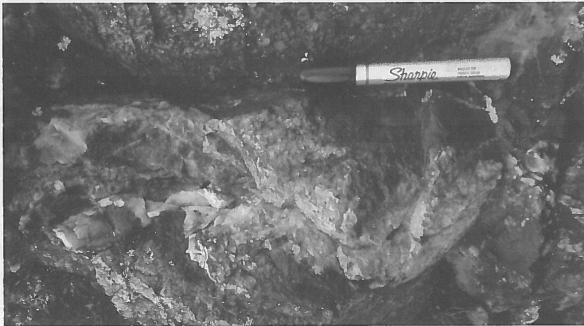
Illustration 4: Close up photo of rust bleed coming off of a discontinuous quartz vein. Yellow to white botryoidal gossan was observed to be quite prominent on some rust bleeds.
