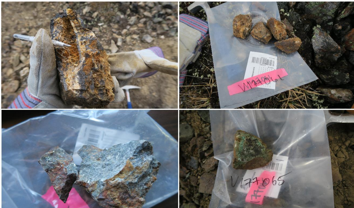
Figure 7: Observed mineralization at the May-Qu prospect. Top left: oxidized, vuggy Fe-Mn altered quartzite retrieved from historic trenches; Top right: intensely oxidized quartz vein, hosted in quartzite (V177061: 0.249g/t Au); Bottom left: Diopside skarn with massive chalcopyrite (5%) and pyrrhotite (2%) mineralization; Bottom right: surface coating of Cu-oxide on diopside skarn (V177065: 2.22g/t Au, 1.065% Cu, 23g/t Ag).
