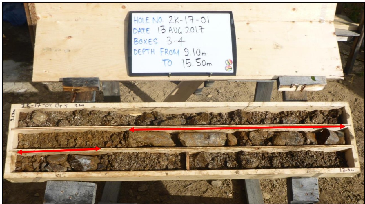
Figure 24: Epithermal quartz veining, down-dip extension of high grade surface sample, DDH 2K17-01
