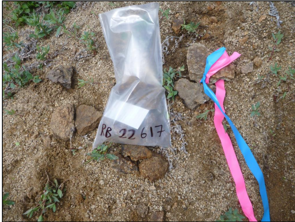
Figure 12: Sample RB22617, 0.597 g/t Au, Epithermal Quartz-Manganese Vein, E of Kenyon Ck placer
