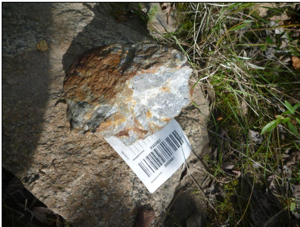
Figure 13: Sample R950461, 4.857 g/t Au; Quartz veins in altered, mineralized granodiorite, H-Grid
