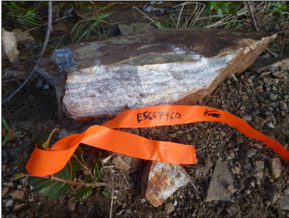
Figure 9: Sample E5667960, banded mesothermal quartz vein, H-Grid area
