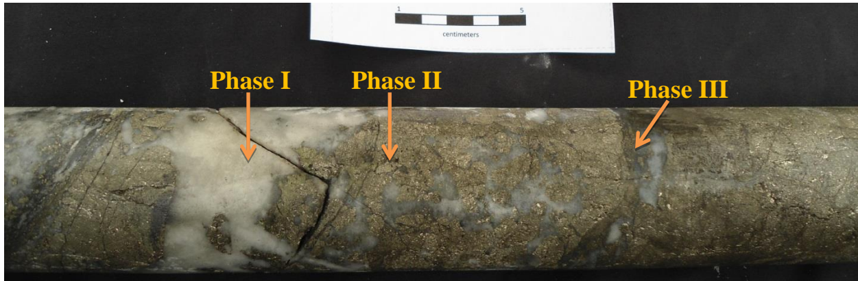
Plate 2: Central BRX Zone drill core highlighting Phases I through III. Quartz and pyrite generally dominate these veins.
