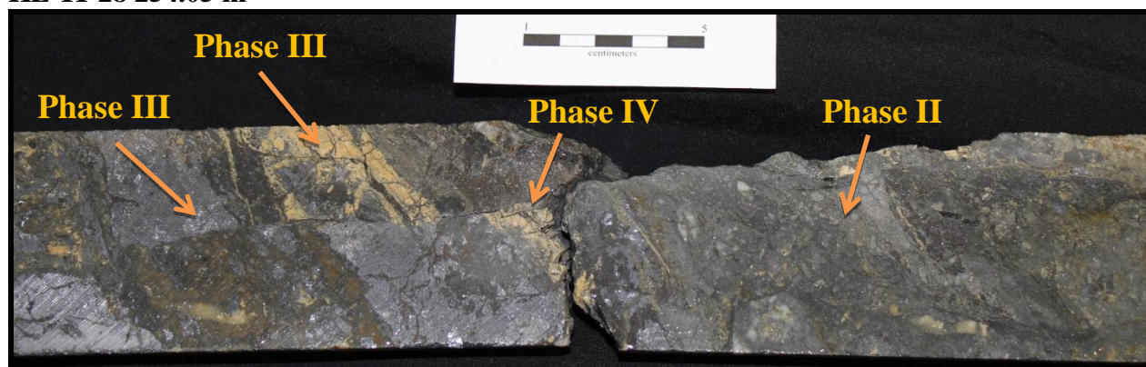
Plate 5: Brecciated galena and ankerite vein cross-cutting smoky quartz/pyrite/arsenopyrite.
