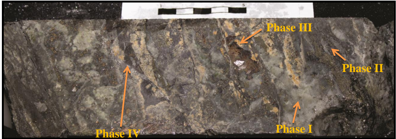
Plate 1: Western BRX Zone intersect highlighting Phases I through IV. Sphalerite and galena are clearly seen in proximity to tan ankerite.
