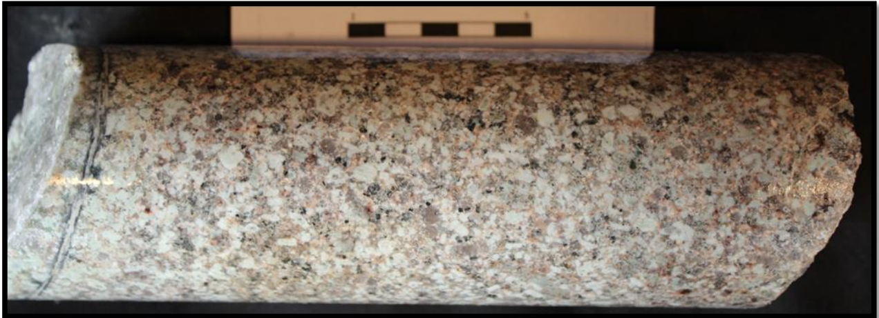
Plate 13: Moderate potassic alteration with secondary biotite.
