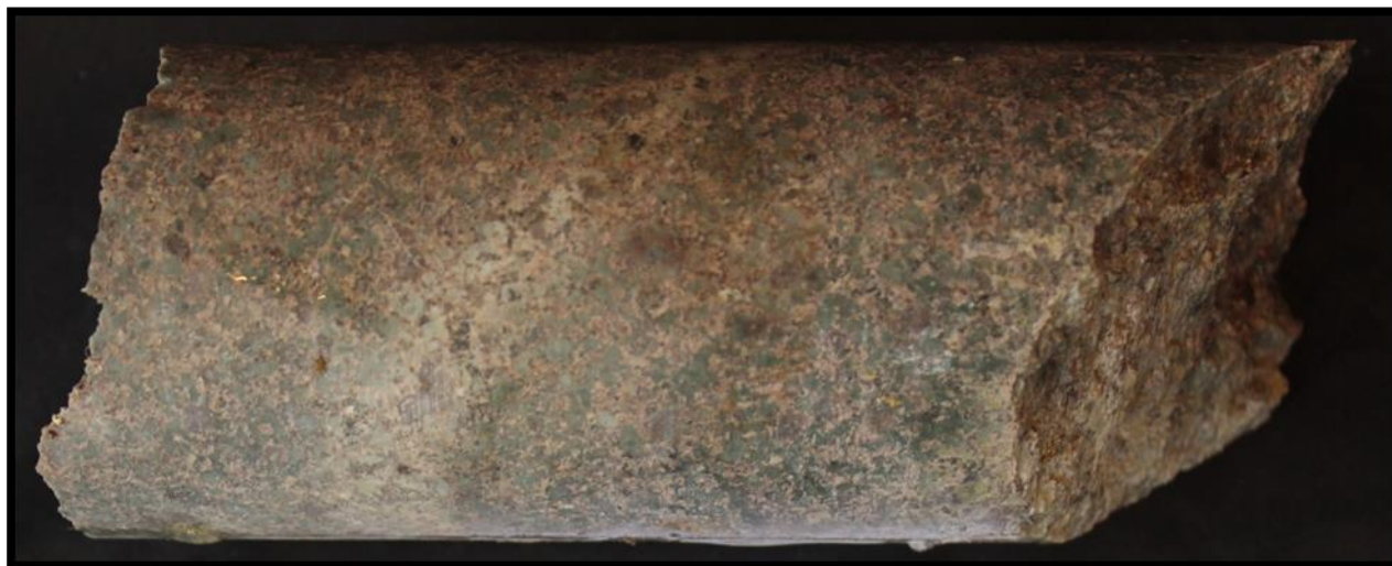
Plate 7: Strong propylitic alteration with weak potassic overprinting.
