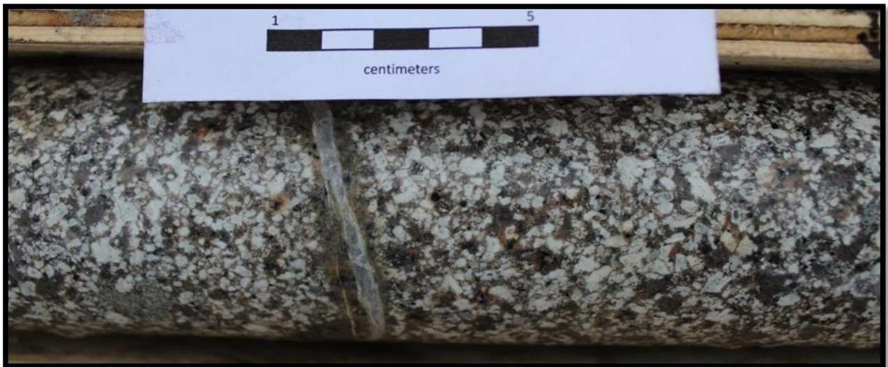
Plate 9: Weak kaolinitic alteration.
