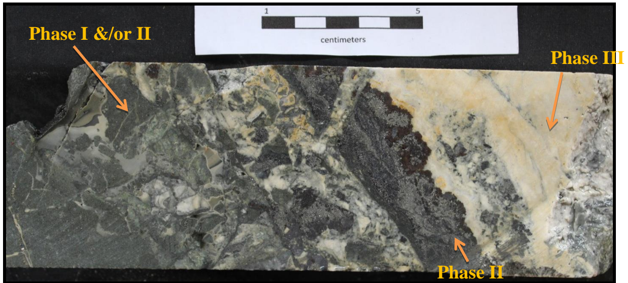
Plate 3: Western Klaza Zone drill core showing fine-grained arsenopyrite veins and breccias with zoned honey brown sphalerite at the margin of a tan ankerite mass.
