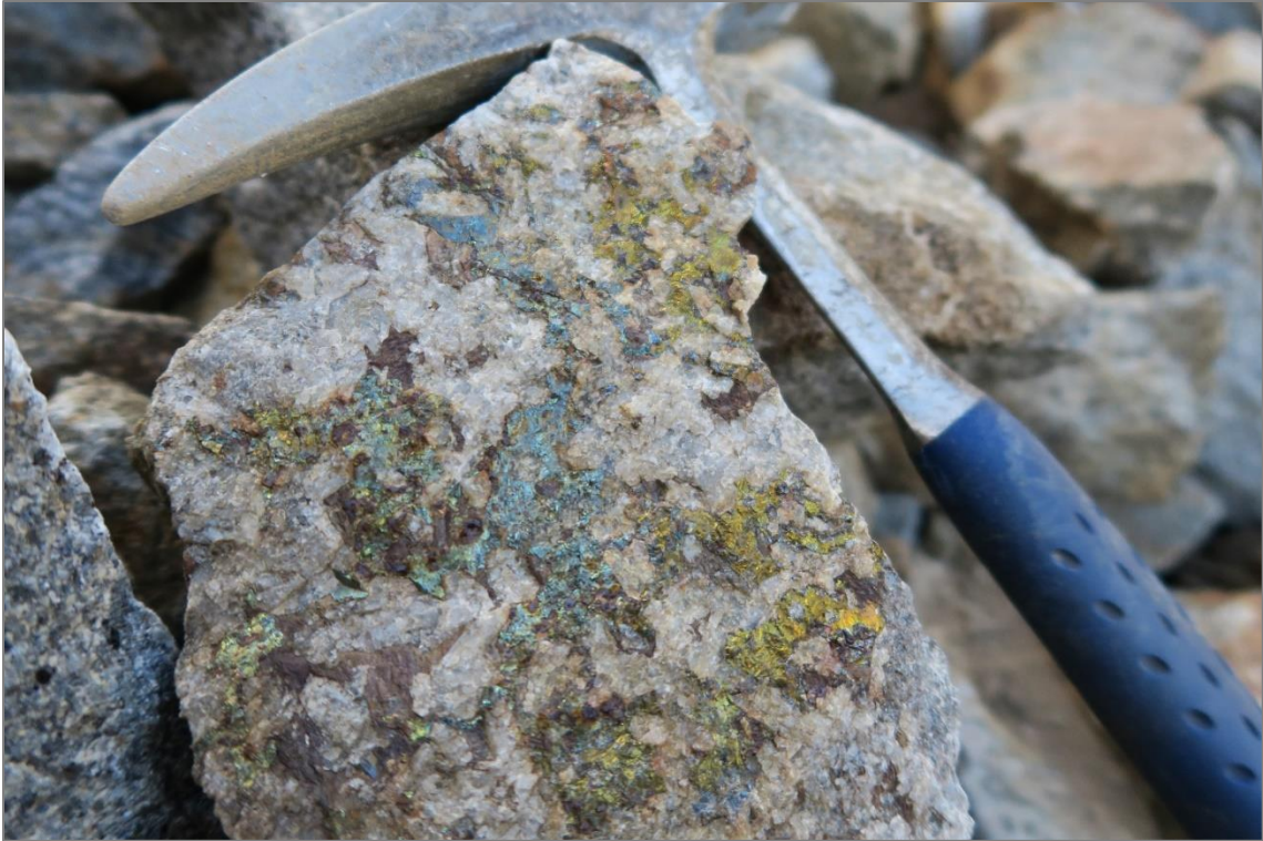
Figure 14: Chalcopyrite-pyrrhotite mineralization on open fracture face of quartz vein from anomalous sheeted-vein complex. Estwing Rock Pick for scale.
