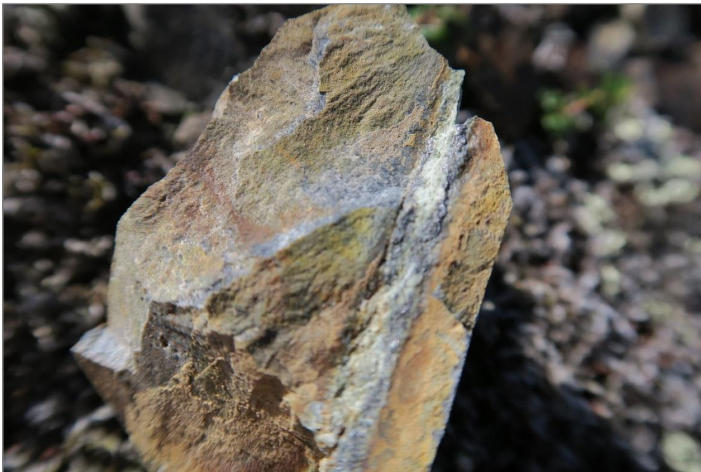
Figure 11: Heavily Fe-weathered siltstone, hosting quartz-arsenopyrite veins proximal to the nonconformity contact with the Nuke intrusion.
