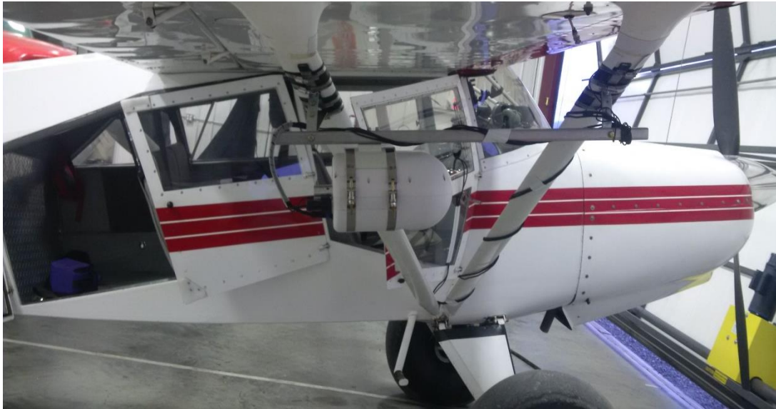
Figure 11: XCAM Mounted to airplane strut.
