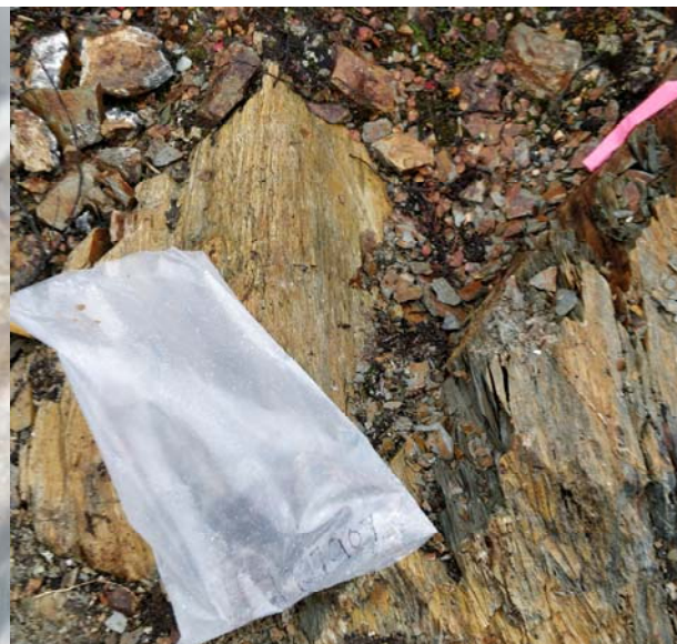
Figure 31: Sample 1907907 Golden Culvert main showing; 1.5m chip of green siliceous phyllite taken between two quartz veins; quartz veinlets throughout; striking 260° azimuth; assay of 1.52gpt Au
