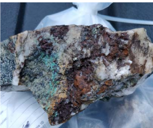
Figure 33: Sample 1907902 Green Dragon showing; quartz vein with disseminated chalcopyrite and malachite stain; assay of 1,751ppm Cu, 4,579ppb Ag.
