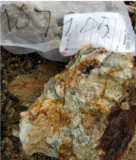
Figure 27: Sample 1907905 Quartz vein in Golden Culvert main showing striking 260° azimuth; euhedral pyrite, sericite; assay of 18.27gpt Au.
