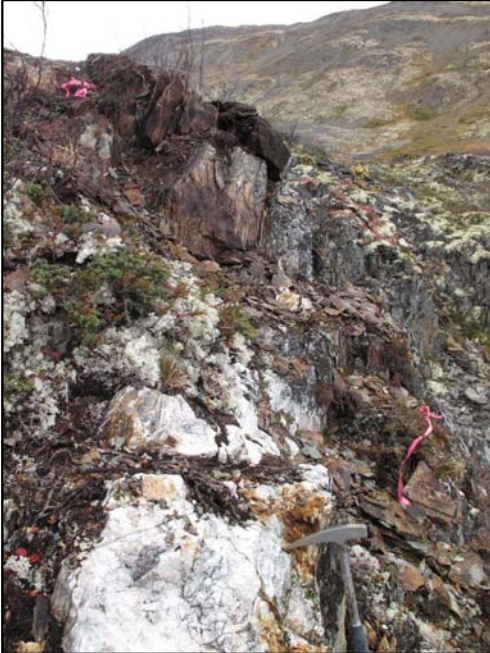
Figure 25: Golden Culvert quartz vein Host rock is sheared, silicified phyllite. Assay of 18.27gpt Au.
