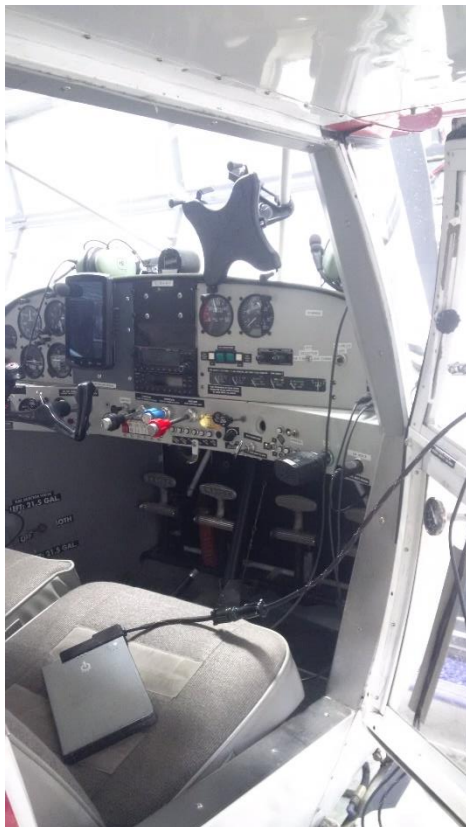
Figure 4. Inside the plane. Note the external battery on the seat, the inverter, and the tablet holder.
