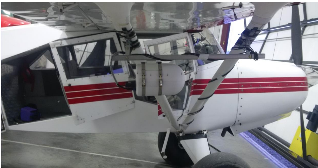
Figure 2. The pod secured the bar attached to the strut.
