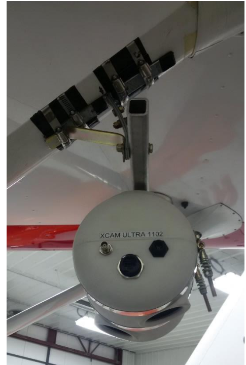
Figure 3. XCam Ultra Pod. Slightly smaller in radius to XCam B but otherwise the small.
