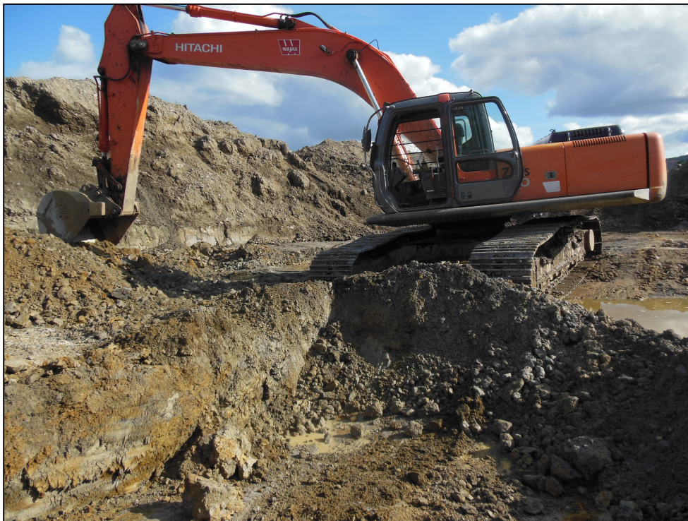
Figure 6. Test pit in altered andesite outcrop at station RH17SM019 (no sulfides or veining of any type).
