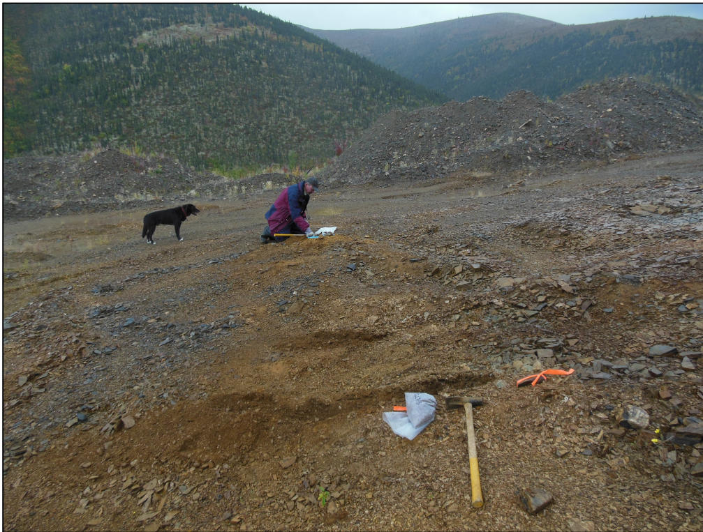
Figure 2. Rock sample 122703 in foreground (2070 ppm As) of muscovite schist with minor iron oxide.
