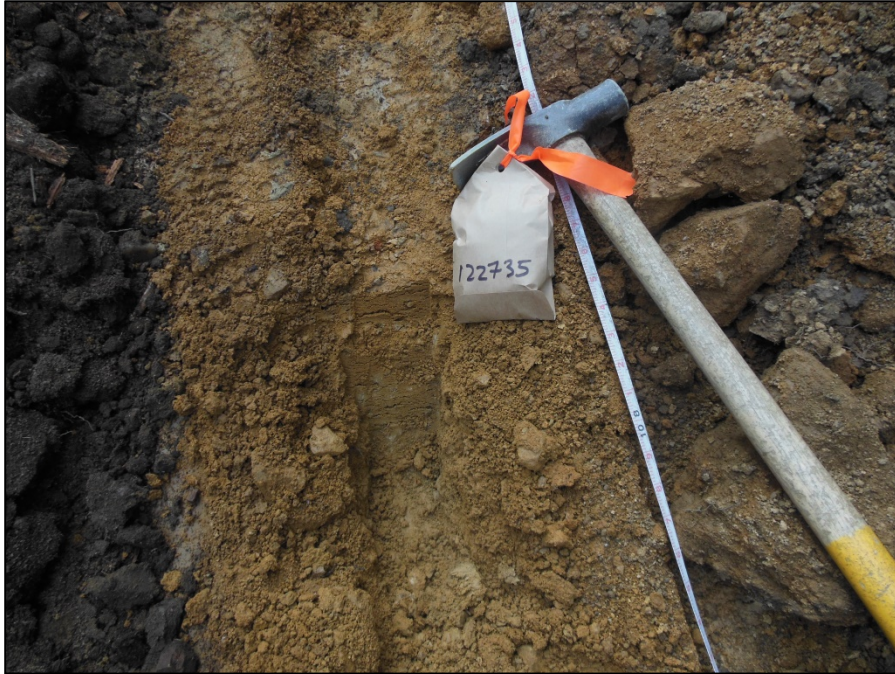
Figure 13. Trench Tr17-2, soil sample 122735 (13.9 ppm Hg) from trench bottom of schist sub-crop, C horizon.
