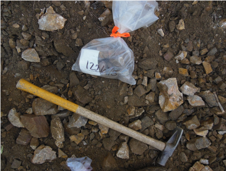
Figure 14. Trench Tr17-3, rock sample 122675 (4.5 ppm Hg) of altered siliceous andesite (?) with mm carbonate + quartz veinlets.
