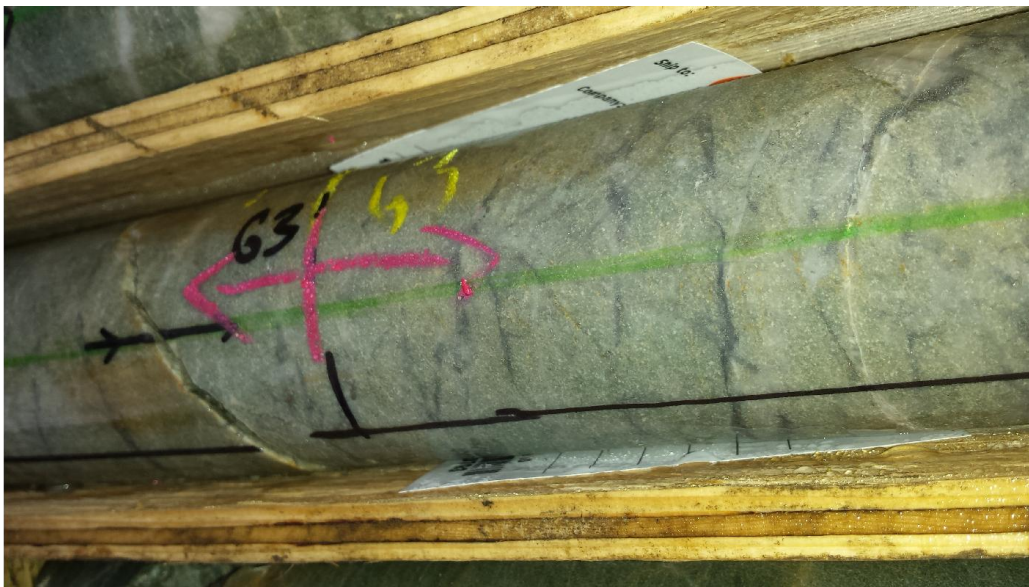
Photo 8: Discordant quartz-arsenopyrite veinlets at 63m (PSGS-16-05).
