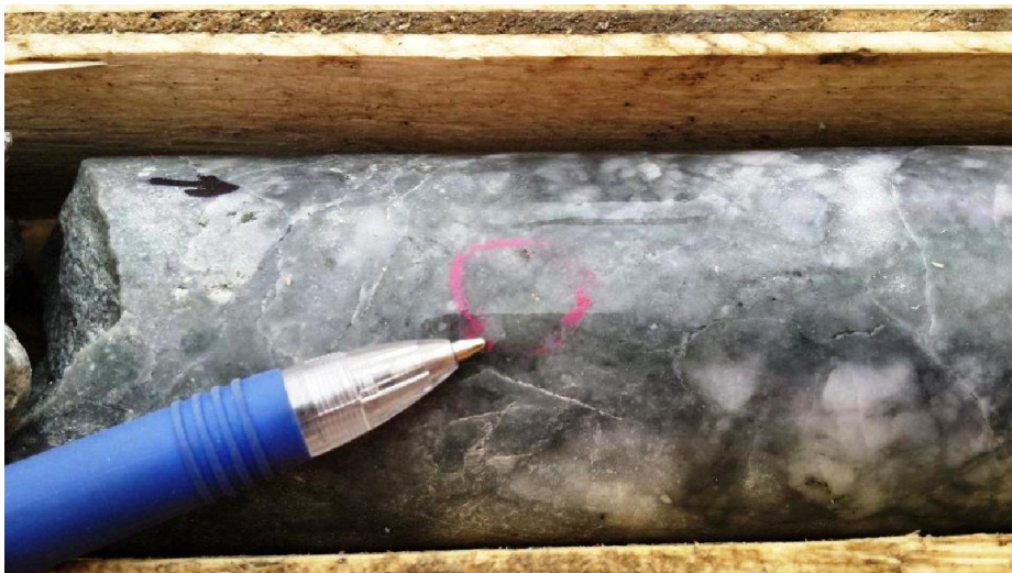
Photo 2: VG in lower hydrothermal breccia unit with arsenopyrite fracture-fill (PSGS-16-01, 50.4m).
