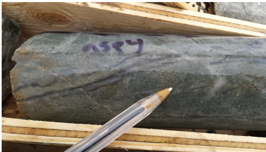
Photo 4: Quartz-arsenopyrite veining at 31.25m (PSGS-16-03).
