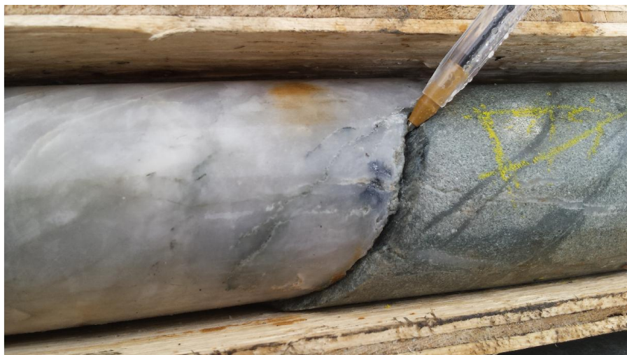
Photo 9: Galena on lower margin of 30cm quartz vein (PSGS-16-07, 74.9m).
