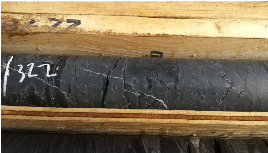
Photo 12: Slumping carbonaceous primary breccia (PSGS-16-10, 322m).
