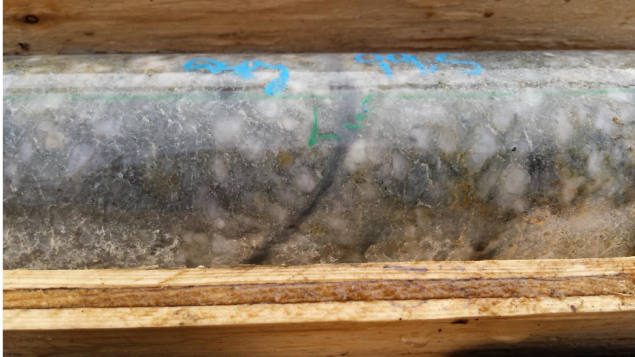
Photo 13: Outlier quartz-arsenopyrite veinlet in silicified grit to pebble conglomerate (PSGS-16-11, 99.5m).
