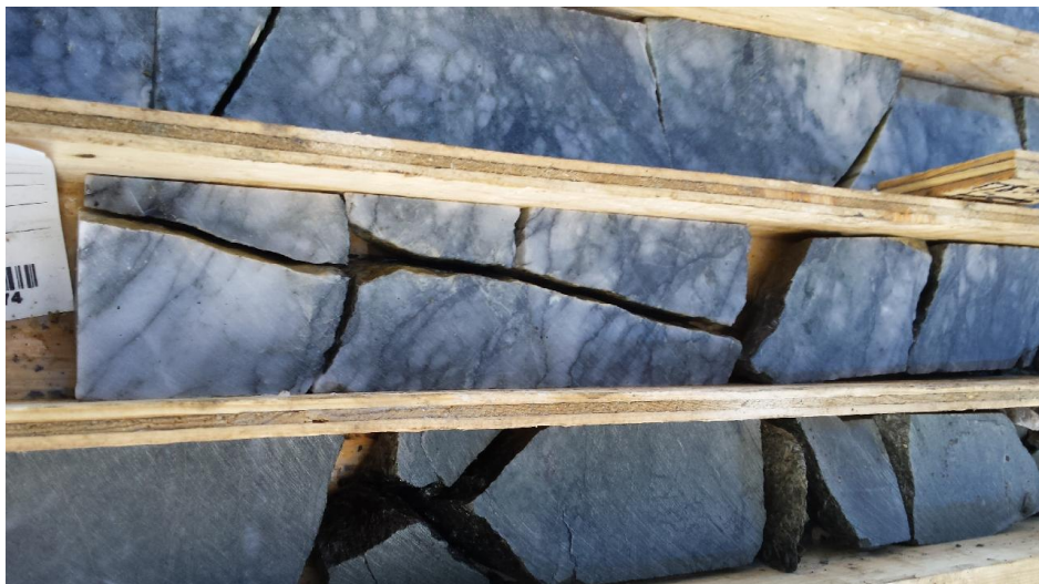
Photo 15: Arsenopyrite in brecciated pebble conglomerate and quartz (PSGS-16-11, 178m).
