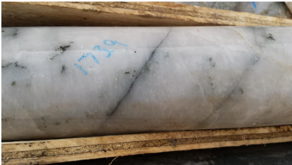
Photo 14: Arsenopyrite fracture-fill in earlier quartz veining (PSGS-16-11, 173.9m).
