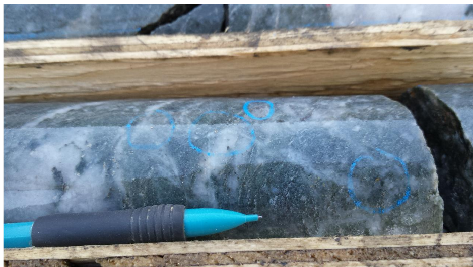
Photo 10: Multiple gold grains in mineralized quartz stockwork (PSGS-16-08, 73.7m)
