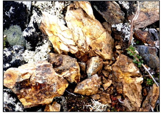
Photo 4: Sample 1353625 – 3508 ppm As, 67.7 ppm Sb, 5.46 ppm Hg, 2.6 ppm Se, 15% Fe →
