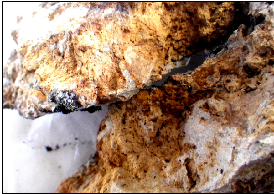
Photo 5: Sample 1353636 – 850.9 ppm As, 138.4 ppm Sb, 3.94 ppm Hg, 3.5 ppm Se
