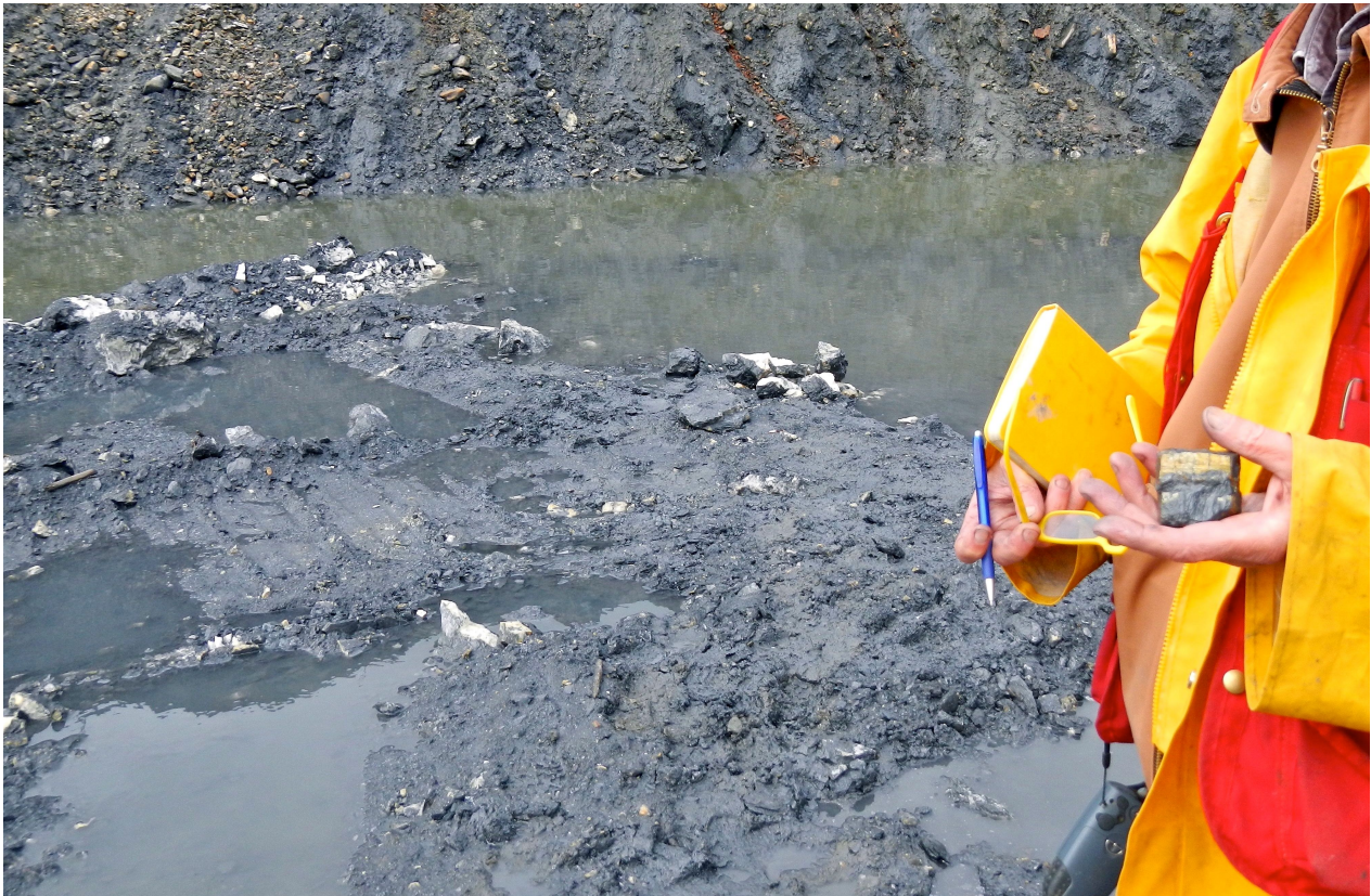
Same structure is observed approx. 3kms north-west at the Last Chance Dredge Pit. “Pyrite Cube” from 2015 examination of Last Chance placer pit bedrock exposure. Visited with permission from the placer operator, Karl Knutsen. The black shale – sulfide – quartz mélange seen at the bedrock base lies below the listwanite “slab” that the dredge (1 st pic of appendix) sits on top of.
