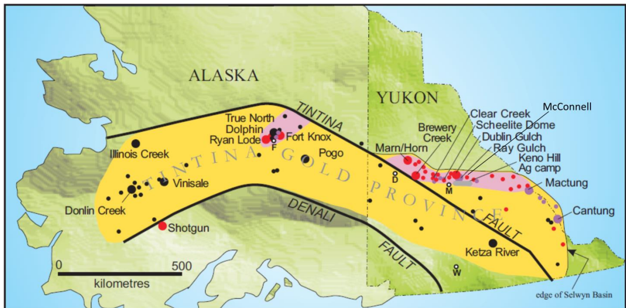
Figure 6.1. Map of the Tintina Gold Province for the Yukon Territory and Alaska. Mineral deposits are shown as large circles, mineral occurrences are shown as small circles. Gold deposits in red dots could be considered under the same genetic model as McConnells Jst. Deposits marked in black dots are not of the same origin, or are ambiguous in origin. Deposits marked in purple are skarn deposits (predominantly W-bearing). Within the TGP is the Tombstone Gold Belt (TGB; marked in pink) which is the major host to gold deposits in the Yukon and Alaska. Mair et al. (2006) suggested ~450 km of post-formation offset along the Tintina Fault, causing displacement of the Fairbanks district. Population centres marked are Whitehorse (W), Mayo (Mayo), Dawson (D) and Fairbanks (F). After Hart (2007).
